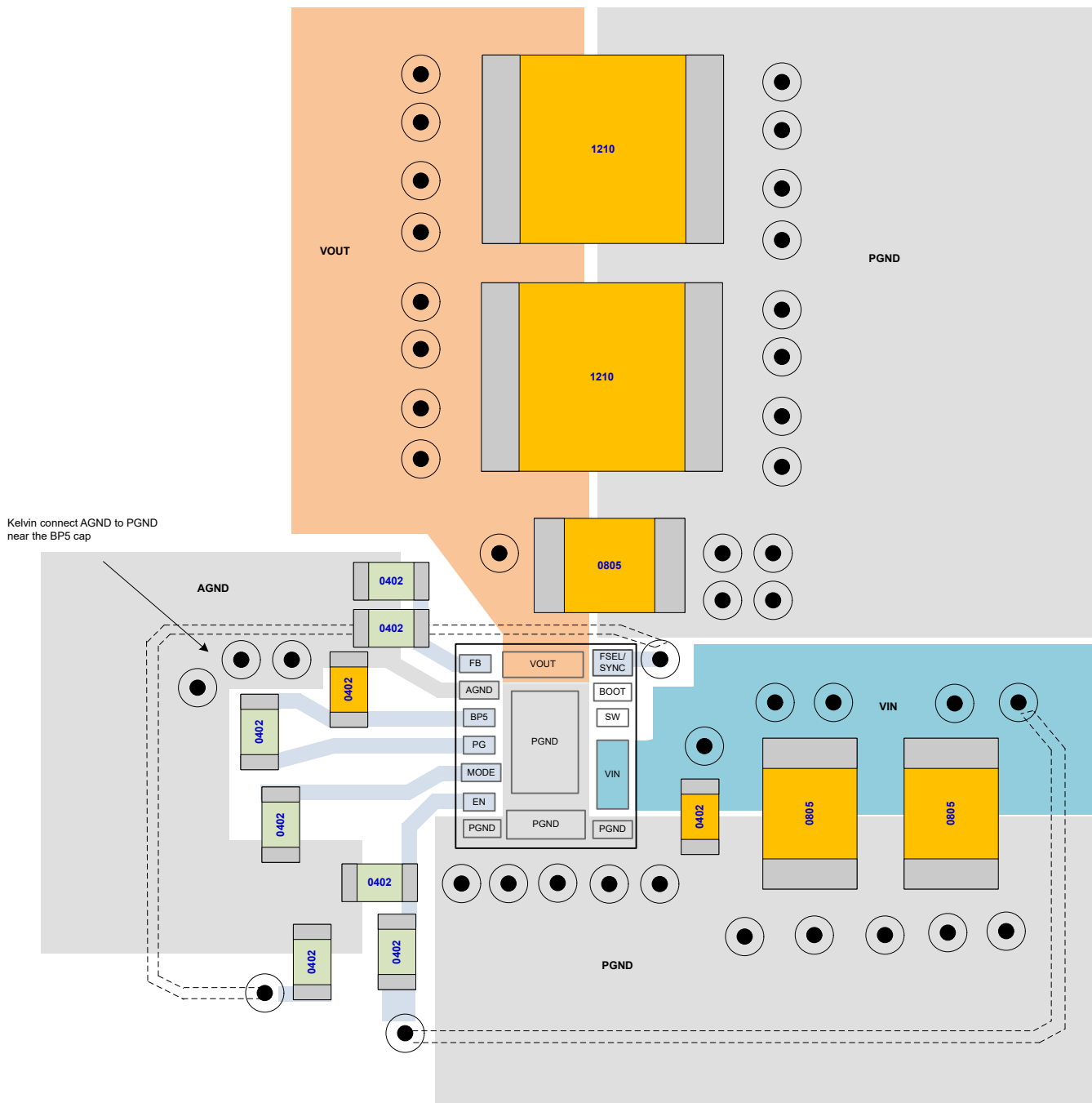
Figure 7-19. Example PCB Layout
