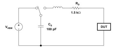
Figure 8-1. HBM ESD Test Circuit
