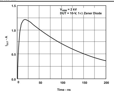
Figure 8-2. Typical HBM Current Waveform
