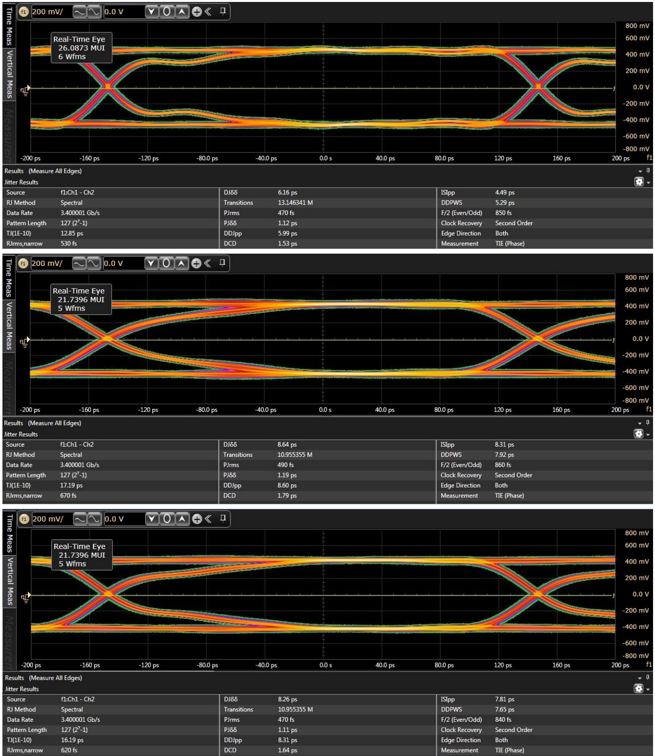
Figure 6-5. Typical eye diagrams at 3.4 Gbps. Top: baseline calibration setup. Middle: through TS3DV642-Q1 Port A. Bottom: through TS3DV642-Q1 Port B.
