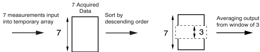
Figure 28. MAV Filter Operation (Patent Pending)
