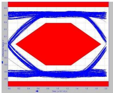
**Figure 30. 2 meter post-channel with TUSB217-Q1 BOOST=1 RX\_SEN=HIGH**
