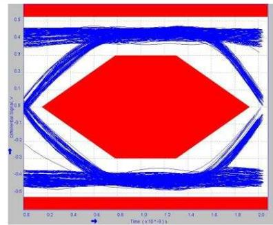
**Figure 29. 2 meter post-channel with TUSB217-Q1 BOOST=1 RX\_SEN=MED**
