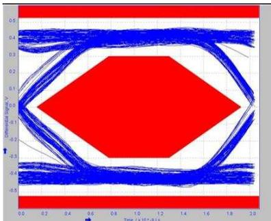
Figure 13. 3 meter pre-channel with TUSB217-Q1 BOOST=0 RX\_SEN=MED
