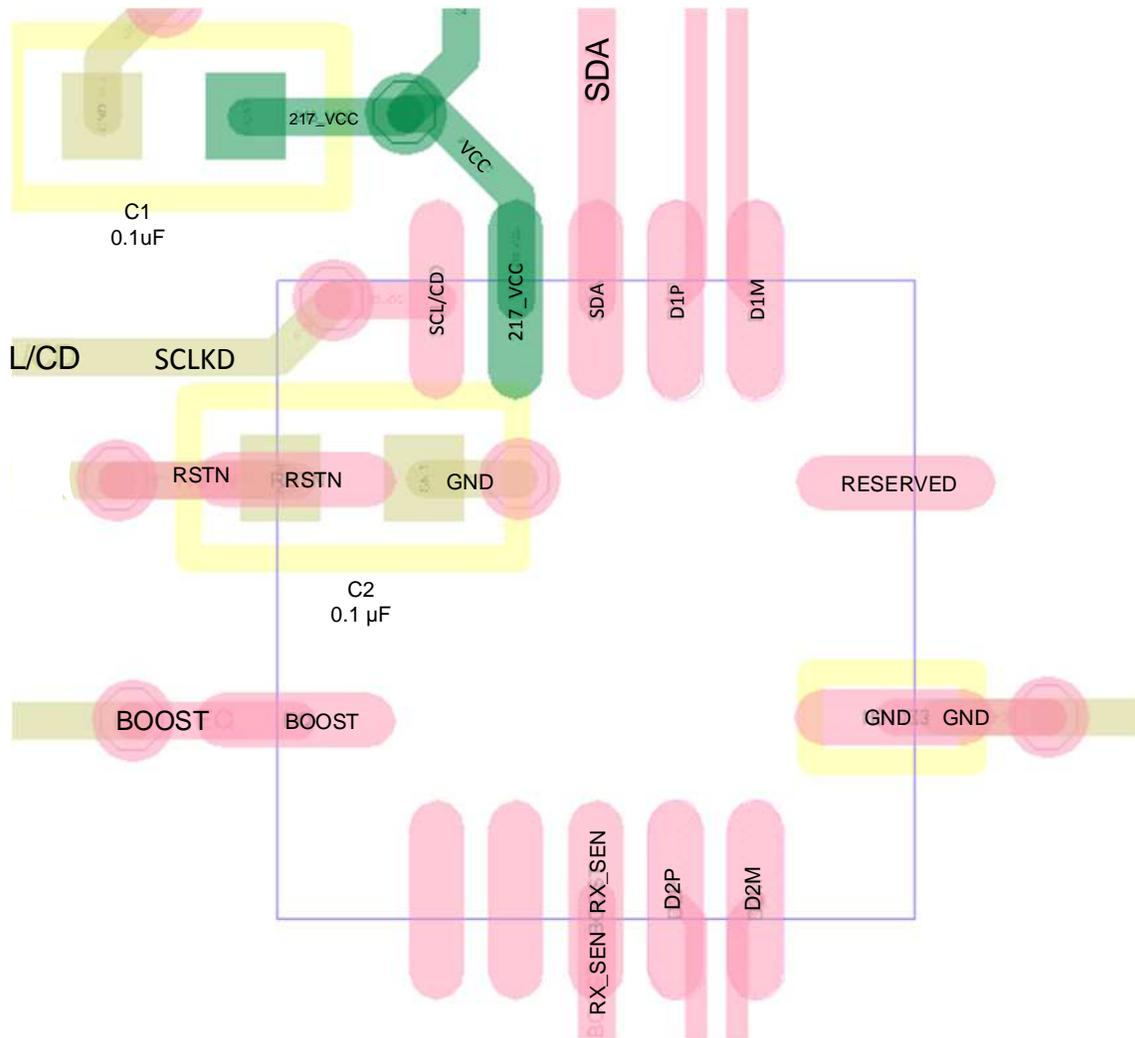
**Figure 34. Layout Example (thermal pad grounding is optional)**
