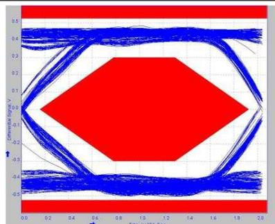
Figure 16. 2 meter pre-channel with TUSB217-Q1 BOOST=1 RX\_SEN=MED
