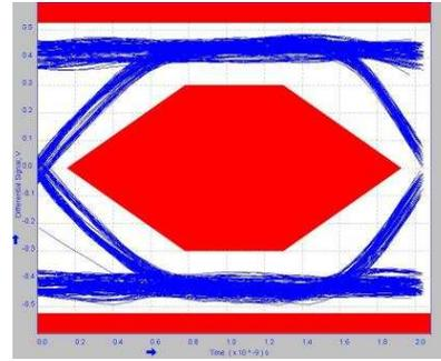
**Figure 27. 1 meter post-channel with TUSB217-Q1 BOOST=0 RX\_SEN=HIGH**
