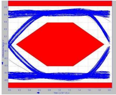
**Figure 26. 1 meter post-channel with TUSB217-Q1 BOOST=0 RX\_SEN=MED**
