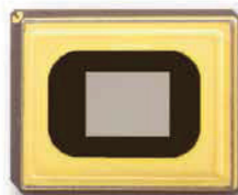
Array diagonal: 0.7" Micromirror array: 1024x768
