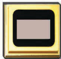
Array diagonal: 0.9" Micromirror array: 2560x1600
