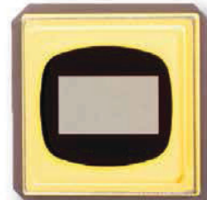
Array diagonal: 0.95" Micromirror array: 1920x1080
