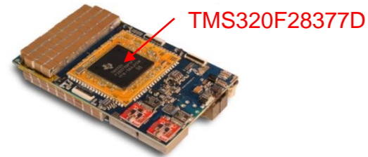
Series stacked energy buffer
