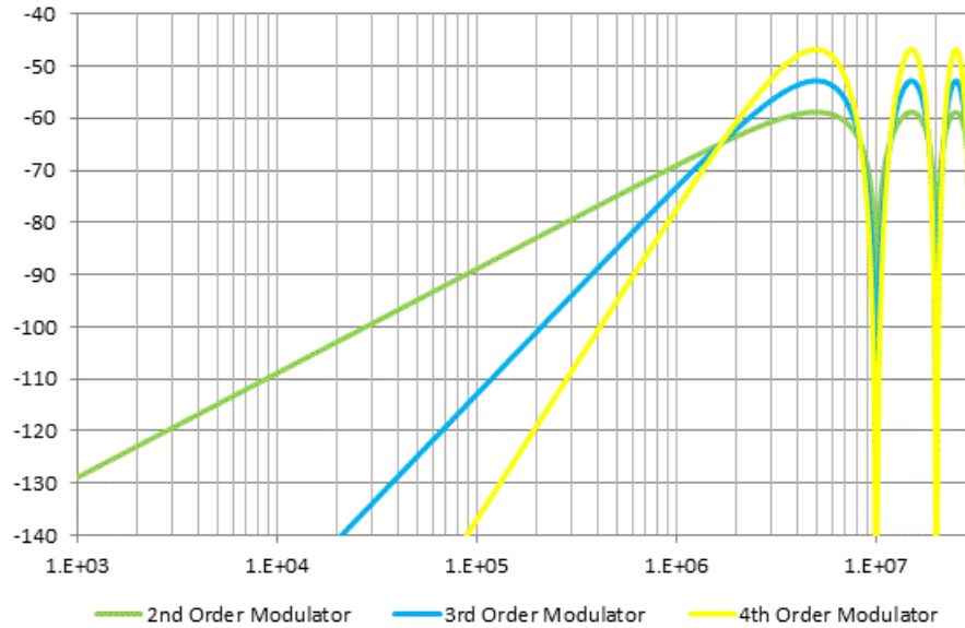
Figure 10.5 Theoretical Delta Sigma Noise for a 10 MHz Phase Detector Frequency
