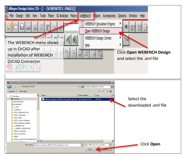
2. Once opened you will see your schematic in OrCAD the same as it appears in WEBENCH online. The files include models and simulation settings. Click on the **Run WEBENCH Simulation Engine** toolbar icon to launch simulation.
