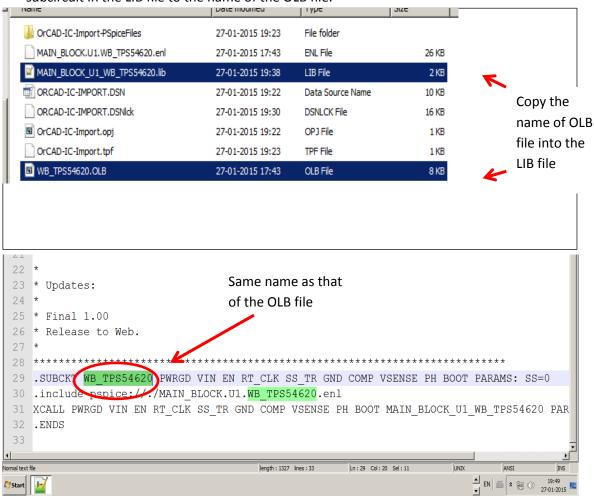
g. Once these changes are made, the next step is to place the part in the schematic editor of OrCAD.
