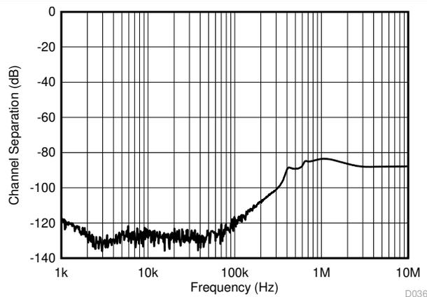
Figure 7-36. Channel Separation
