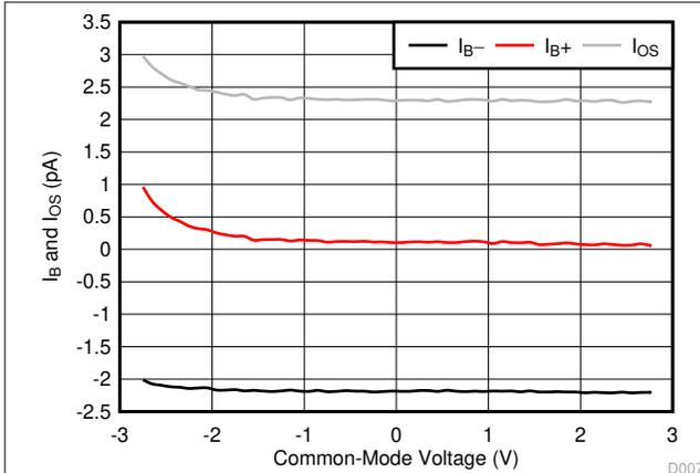
**Figure 7-7.  $I_B$  and  $I_{OS}$  vs Common-Mode Voltage**
