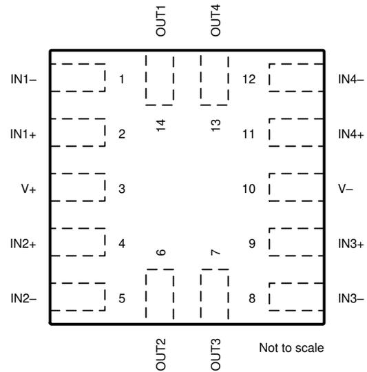
**Figure 6-12. TLV9004 RUC Package 14-Pin X2QFN Top View**
