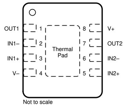
A. Connect thermal pad to V-.
