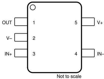
**Figure 6-1. TLV9001 DBV, TLV9001T DCK Package
