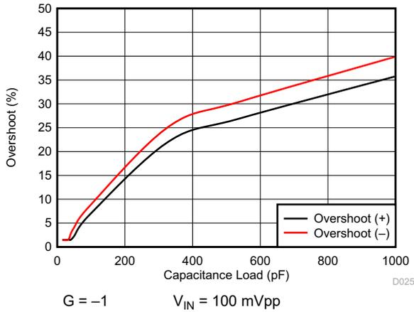
**Figure 7-25. Small Signal Overshoot vs Capacitive Load**
