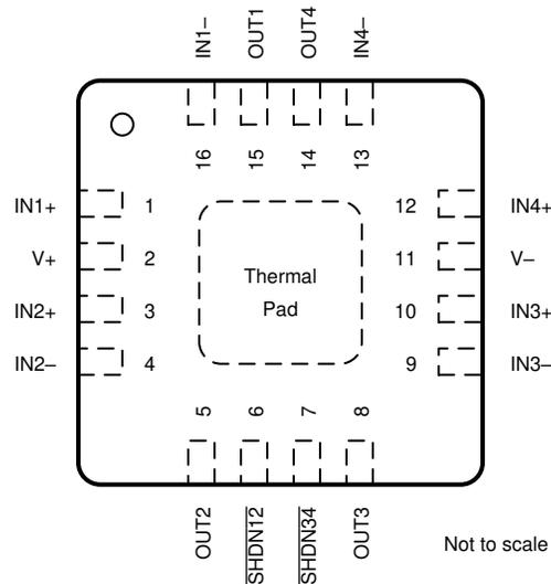
A. Connect thermal pad to V-.
