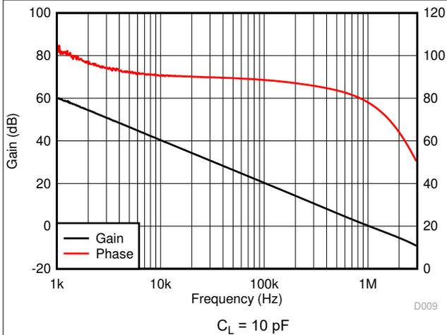
**Figure 7-9. Open-Loop Gain and Phase vs Frequency**
