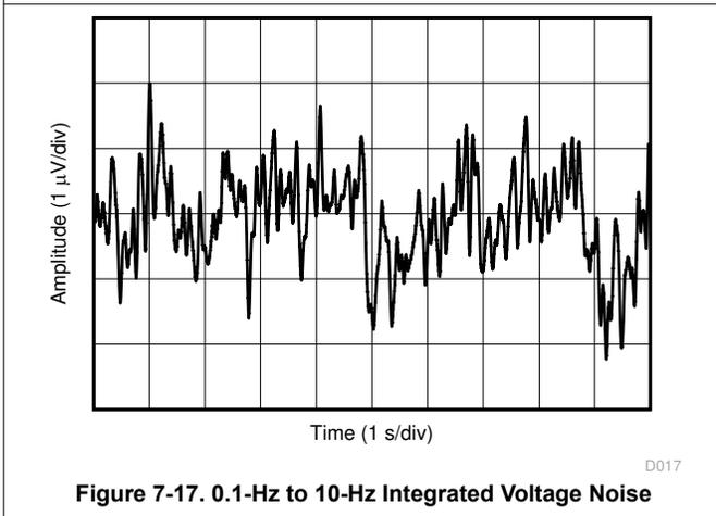
Figure 7-17. 0.1-Hz to 10-Hz Integrated Voltage Noise
