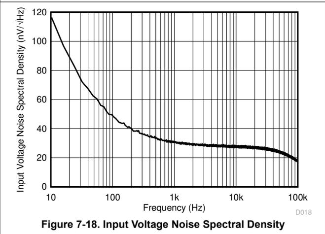
Figure 7-18. Input Voltage Noise Spectral Density
