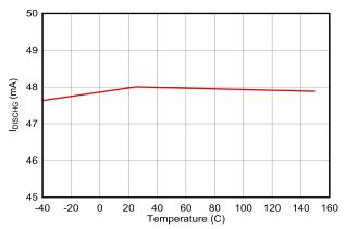
Figure 6-34. V<sub>BUS</sub> Discharge Current vs Temperature
