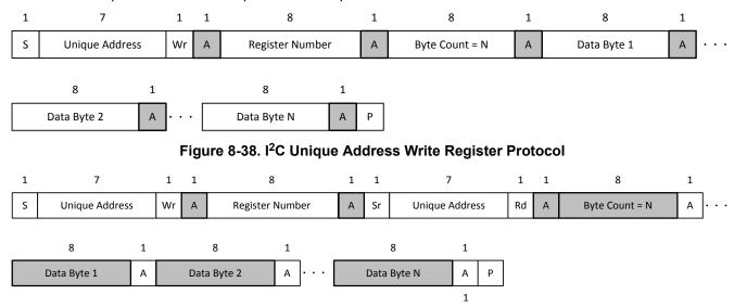
Figure 8-39. I<sup>2</sup>C Unique Address Read Register Protocol
