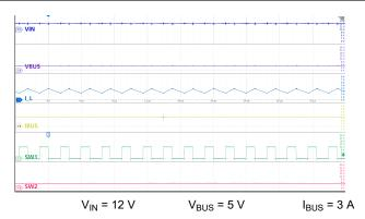
Figure 9-20. Buck Mode: nominal V<sub>IN</sub>, 3 A Load
