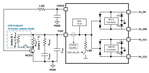
Figure 8-6. Example Circuit to Enable USB Endpoint Firmware Update Mode
