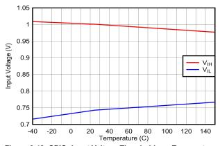
Figure 6-48. GPIO: Input Voltage Thresholds vs Temperature
