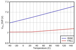
Figure 6-41. Type-C Cable Detect & V<sub>CONN</sub>: Over-voltage Protection Thresholds vs Temperature
