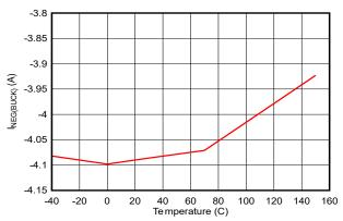
Figure 6-21. Buck Negative Current Limit vs Temperature
