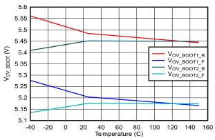
Figure 6-23. BOOTx OVP vs Temperature
