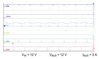
Figure 9-24. Buck-Boost Mode:  $V_{IN} = V_{BUS}$ , 3 A Load
