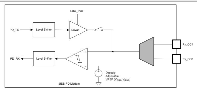
Figure 8-22. USB-PD BMC TX/Rx Block Diagram
