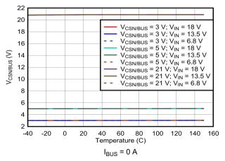
Figure 6-33. Buck-boost Output Voltage Regulation vs
