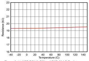
Figure 6-44. USB BC1.2: DM to AGND 20 k $\Omega$  Resistance,  $R_{DM\_DWN\_20k}$
