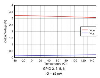
Figure 6-47. GPIO: Output Voltage vs Output Current and Temperature
