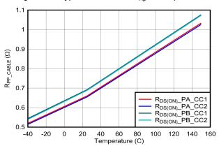
Figure 6-39. V<sub>CONN</sub> Power Path: R<sub>DS(ON)</sub> vs Temperature
