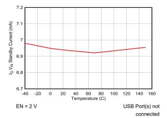
Figure 6-2. IQ VIN Standby Current vs Temperature
