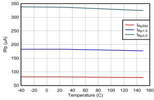
Figure 6-37. Type-C Cable Detect:  $I_{Rp}$  vs Temperature
