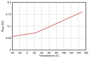
Figure 6-38. Type-C Cable Detect: R<sub>SNK</sub> vs Temperature
