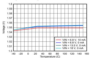
Figure 6-12. LDO\_1V5 vs  $V_{\mbox{\scriptsize IN}}$  and Temperature
