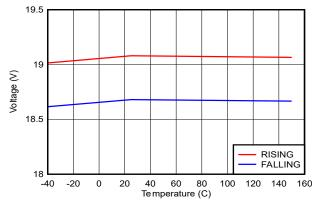
Figure 6-7. V<sub>IN(OVP)</sub> vs Temperature
