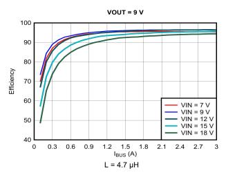
Figure 9-7. Efficiency vs Output Current ( $I_{OUT}$ ),  $V_{OUT} = 9 \text{ V}$
