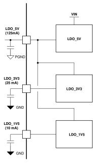
Note: LDO\_5V max regulation current includes LDO\_3V3 (25 mA) and LDO\_1V5 (10 mA)
