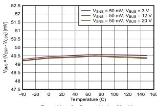
Target V<sub>SNS</sub> for Current Limit = 50 mV Current Limiting Engaged
