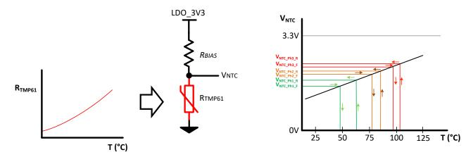
Figure 8-44. TMP61 PTC Response Curve
