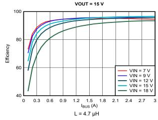
Figure 9-9. Efficiency vs Output Current ( $I_{OUT}$ ),  $V_{OUT} = 15 \text{ V}$
