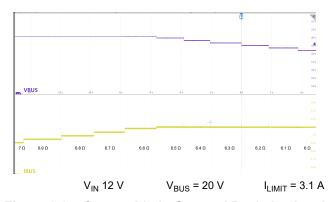
Figure 9-34. Current Limit: Stepped Resistive Load
