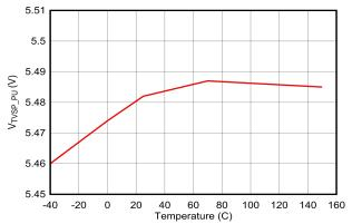
Figure 6-14. V<sub>TVSP\_PU</sub> vs Temperature
