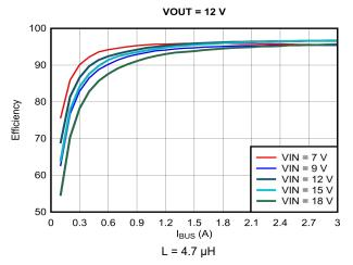
Figure 9-8. Efficiency vs Output Current ( $I_{OUT}$ ),  $V_{OUT} = 12 \text{ V}$
