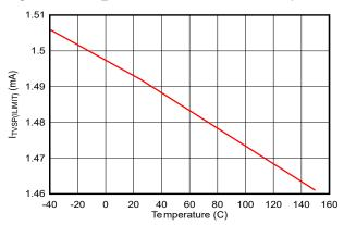
Figure 6-15. I<sub>TVSP(ILIMIT)</sub> vs Temperature
