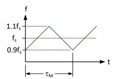
Figure 8-13. Dithering Using Triangular Waveform Modulation
