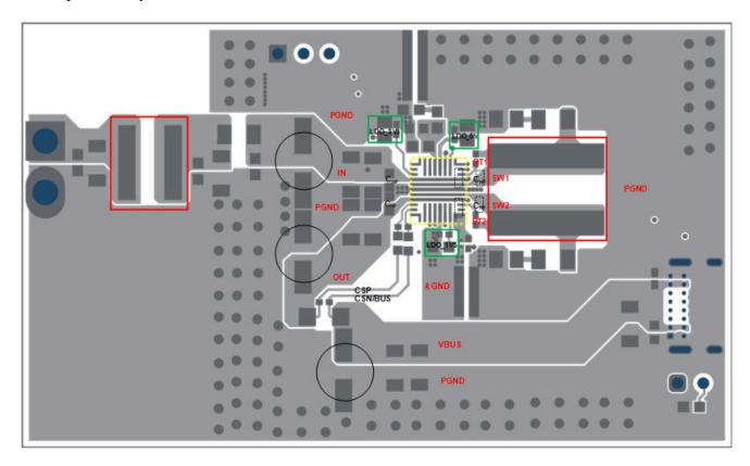
Figure 9-39. TPS25772-Q1 Power Stage Layout
