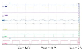
Figure 9-25. Buck-Boost Mode: Nominal  $V_{\text{IN}}$ , No Load
