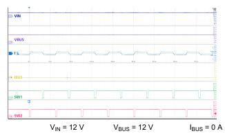
Figure 9-22. Buck-Boost Mode:  $V_{IN} = V_{BUS}$ , No Load
