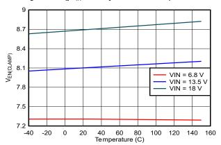
Figure 6-4. EN Clamp Voltage vs Temperature
