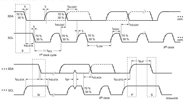
Figure 7-1. I<sup>2</sup>C Target Interface Timing
