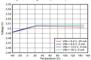
Figure 6-10. LDO\_3V3 vs  $V_{\text{IN}}$  and Temperature
