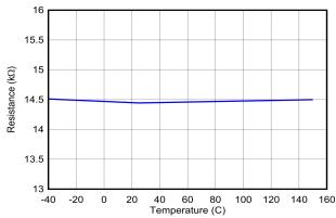
Figure 6-43. USB BC1.2: DM to AGND 15 k $\Omega$  Resistance,  $R_{DM\_DWN\_15k}$
