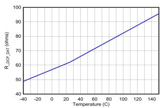
Figure 6-42. USB BC1.2: DP to DM Shorting Resistance,  $R_{\mbox{\scriptsize DCP\_DAT}}$
