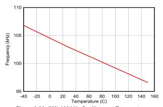
Figure 6-36. (M0) 100 kHz Oscillator vs Temperature
