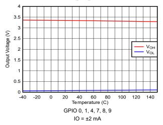
Figure 6-46. GPIO: Output Voltage vs Output Current and Temperature
