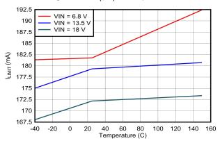
Figure 6-9. LDO\_5V Current Limit vs  $V_{\text{IN}}$  and Temperature
