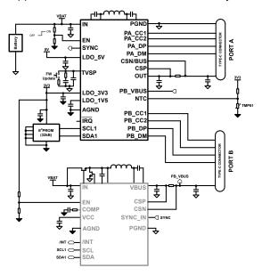
Figure 9-1. Simplified Dual USB PD Charger
