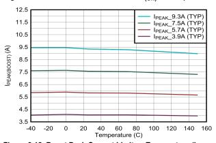
Figure 6-18. Boost Peak Current Limit vs Temperature (lower settings)
