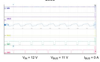
Figure 9-23. Buck-Boost Mode: VIN ≩ VBUS, No Load
