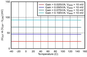
Figure 6-29. Cable Voltage Droop Compensation vs Temperature
