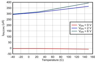
Figure 6-5. EN Leakage Current vs Temperature
