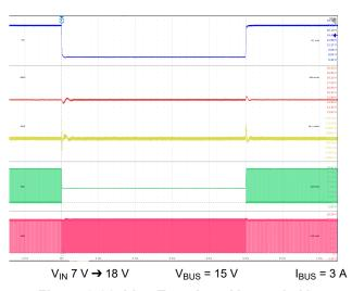
Figure 9-36. Line Transient: V<sub>BUS</sub> = 15 V
