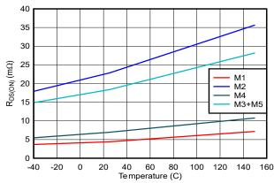
Figure 6-16. Buck-Boost Power FET RDS<sub>(ON)</sub> vs Temperature
