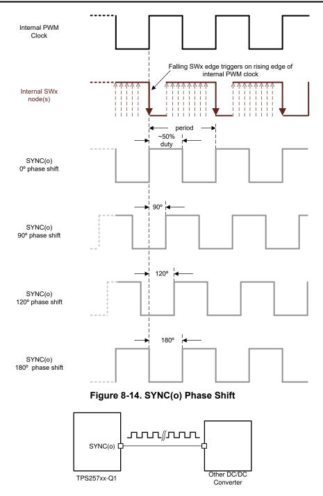
Figure 8-15. Using SYNC(o) to drive external DC/DC Converter
