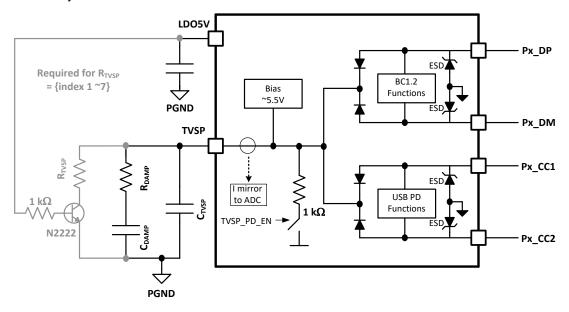
Figure 8-5. R<sub>TVSP</sub> Circuit Configuration
