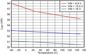
Figure 6-11. LDO\_3V3 Current Limit vs V<sub>IN</sub> and Temperature
