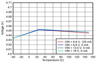
Figure 6-8. LDO\_5V vs V<sub>IN</sub> and Temperature
