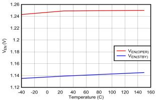
Figure 6-3. ENABLE/UVLO Thresholds vs Temperature
