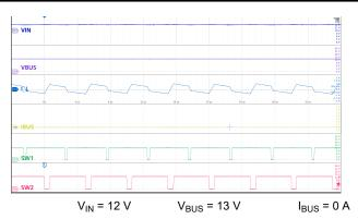
Figure 9-21. Buck-Boost Mode: V<sub>IN</sub> ≨ V<sub>BUS</sub>, No Load
