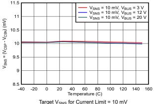
Target V<sub>SNS</sub> for Current Limit = 10 mV Current Limiting Engaged
