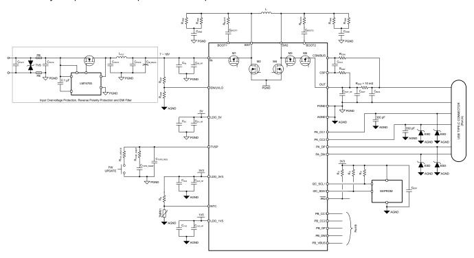
Figure 9-3. TPS25772-Q1 Application Schematic
