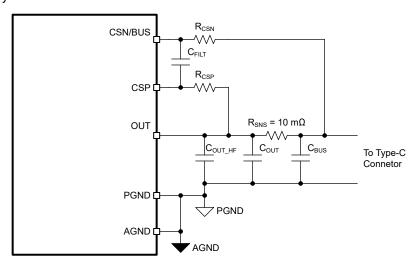
Figure 9-5. Current Sense Amplifier: RC Filter Components
