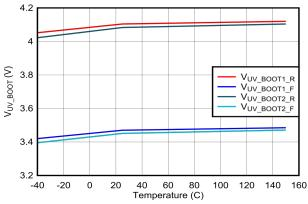
Figure 6-22. BOOTx UVLO vs Temperature
