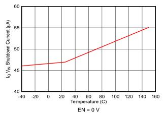
Figure 6-1. I<sub>Q</sub> V<sub>IN</sub> Shutdown Current vs Temperature
