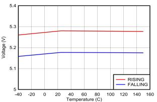
Figure 6-6. V<sub>IN(UVLO)</sub> vs Temperature
