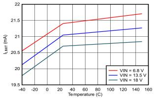
Figure 6-13. LDO\_1V5 Current Limit vs V<sub>IN</sub> and Temperature
