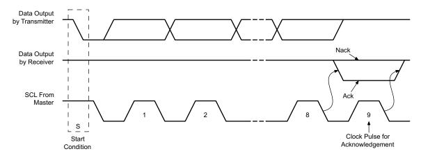
Figure 8-37. I<sup>2</sup>C Acknowledgment
