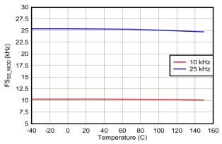
Figure 6-25. f<sub>SW</sub> Dither Modulation Frequency vs Temperature
