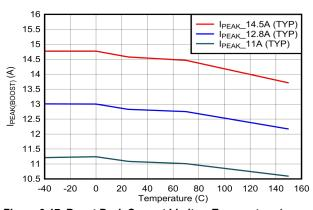
Figure 6-17. Boost Peak Current Limit vs Temperature (upper settings)
