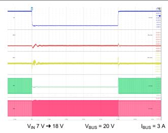
Figure 9-35. Line Transient: V<sub>BUS</sub> = 20 V
