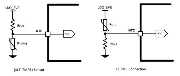
Figure 8-42. Thermistor Connections (a) PTC, (b) NTC
