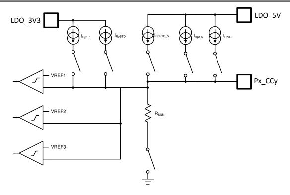
Figure 8-27. Plug and Orientation Detection Block
