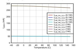
Figure 6-40. V<sub>CONN</sub> Power Path: Current Limit vs Temperature
