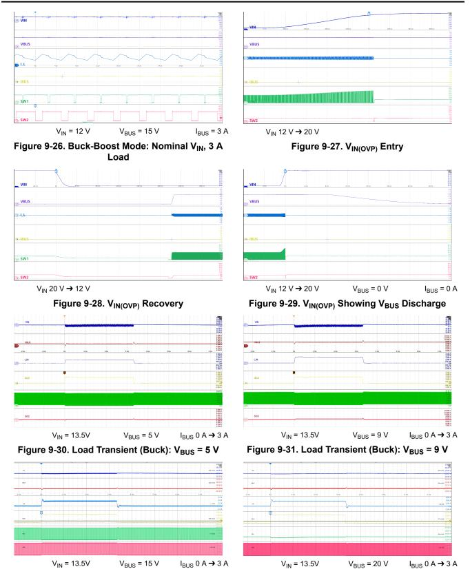
Figure 9-32. Load Transient (Buck-Boost): V<sub>BUS</sub> = Figure 9-33. Load Transient (Boost): V<sub>BUS</sub> = 20 V
