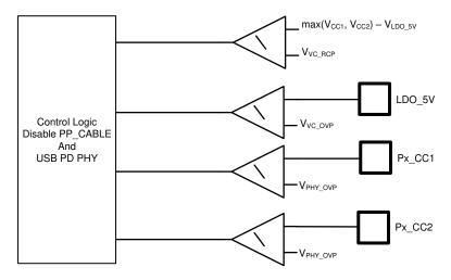
Figure 8-29. Over-voltage and Reverse Current Protection
