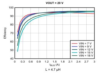
Figure 9-10. Efficiency vs Output Current ( $I_{OUT}$ ),  $V_{OUT} = 20 \text{ V}$
