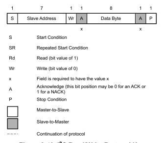
Figure 8-40. I<sup>2</sup>C Read/Write Protocol Key
