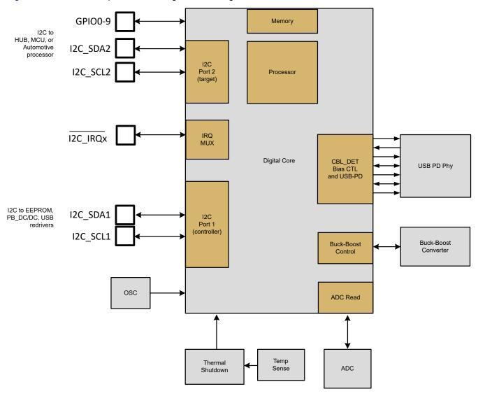
Figure 8-41. Digital Core Simplified Block Diagram
