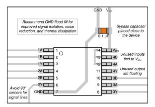
Figure 8-3. Example Layout for the SN74AHCT00Q-Q1
