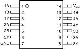
Figure 4-2. D or PW Package, 14-Pin SOIC or TSSOP (Top View)
