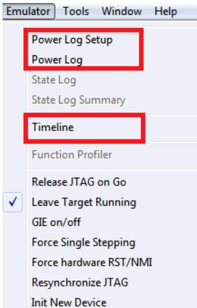
**Figure 3-14. Emulator Pulldown Menu With EnergyTrace-Related Functions**
