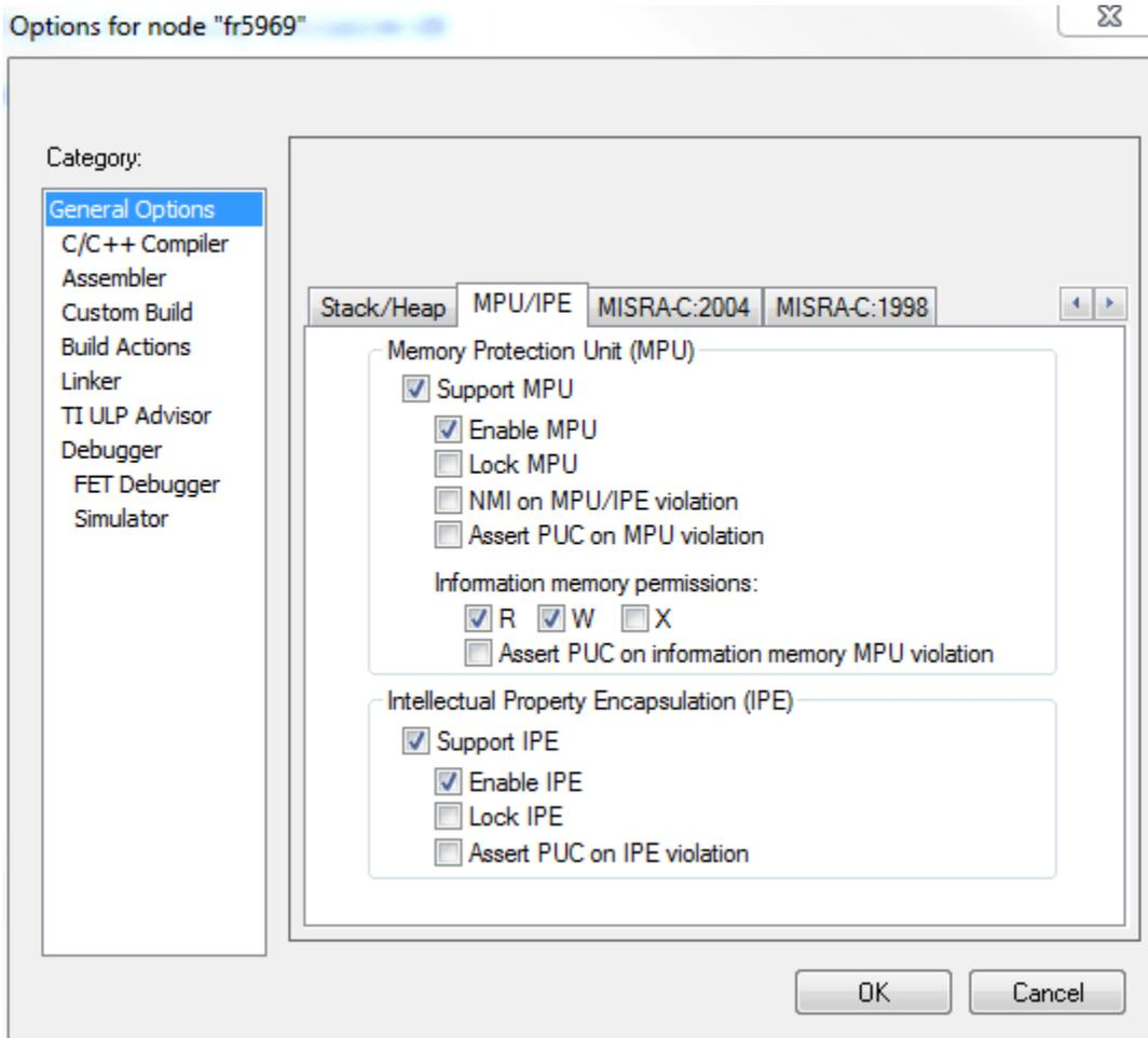
Figure 4-1. MPU Configuration Dialog
