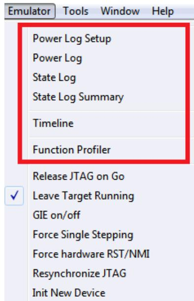
**Figure 3-4. Emulator Pulldown Menu With EnergyTrace++-Related Functions**
