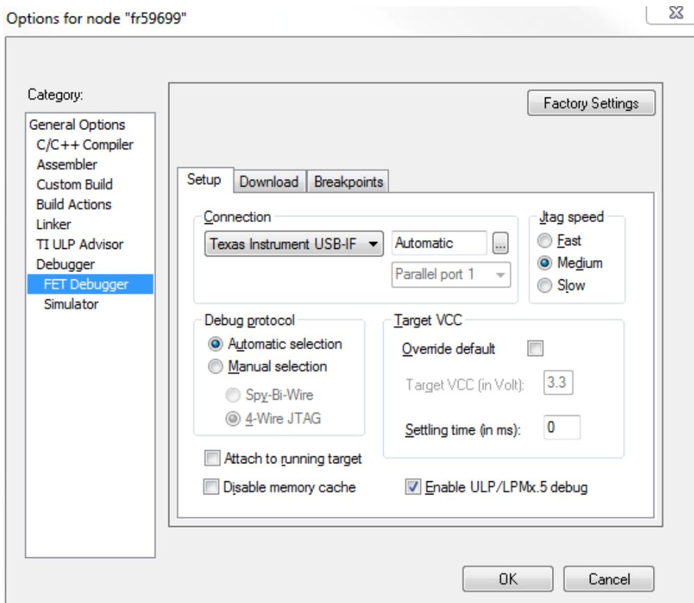
**Figure 2-4. Enable Ultra-Low-Power Debug Mode**
