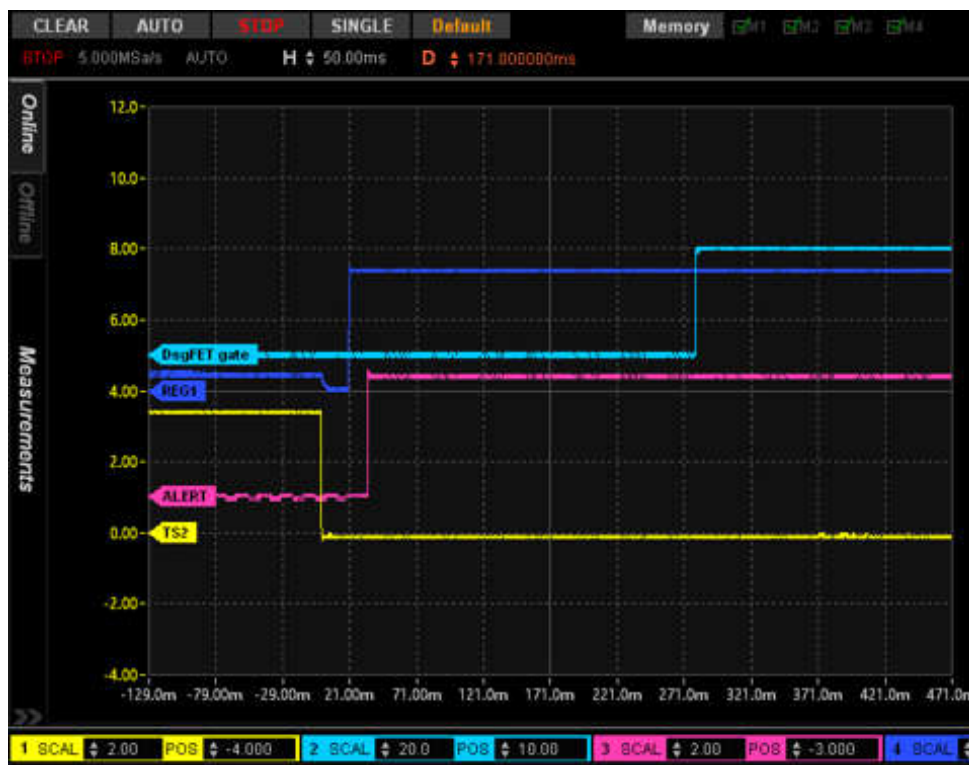
Figure 8-6. Startup Sequence Using [FASTADC] = 1 , with the [INITCOMP] Flag Displayed on the ALERT Pin
