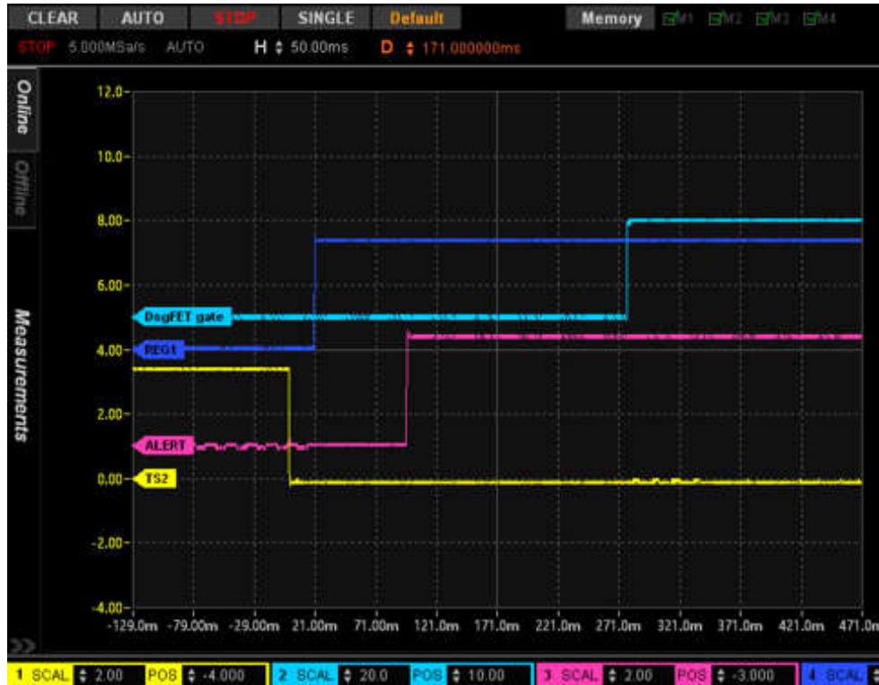
Figure 8-7. Startup Sequence Using [FASTADC] = 0 , with the [FULLSCAN] Flag Displayed on the ALERT Pin
