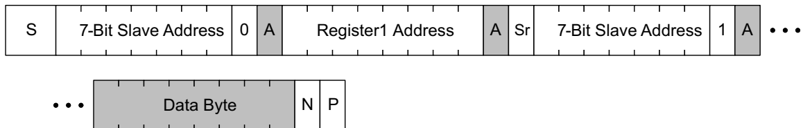
Figure 30. I 2 C Read Data Format
