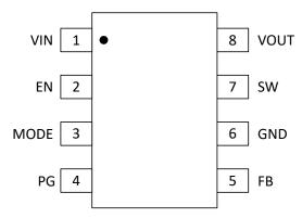
Figure 6-1. DRL Package 8-Pin SOT583 Top View
