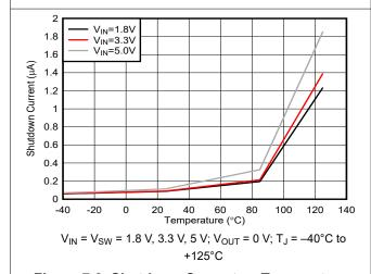
Figure 7-9. Shutdown Current vs Temperature
