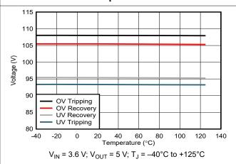
Figure 7-10. PGOOD threshold vs Temperature
