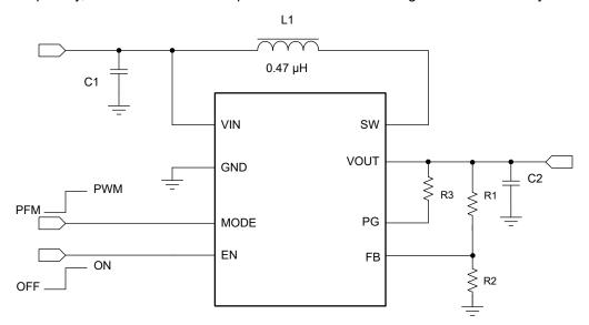
Figure 9-1. Li-ion Battery to 5-V Boost Converter
