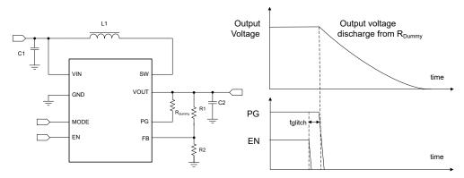
Figure 8-1. Implement Output Discharge by PG function
