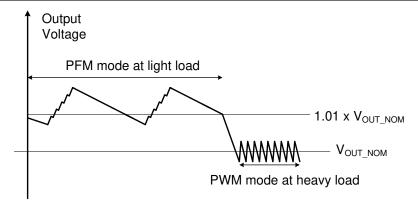
Figure 8-2. Output Voltage in PWM Mode and PFM Mode
