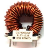
100-kHz CCM PFC inductor (1000 W)
