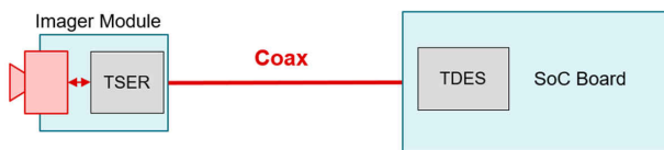
Figure 1. Transporting video over fewer cables without compression using V3Link SerDes devices.
