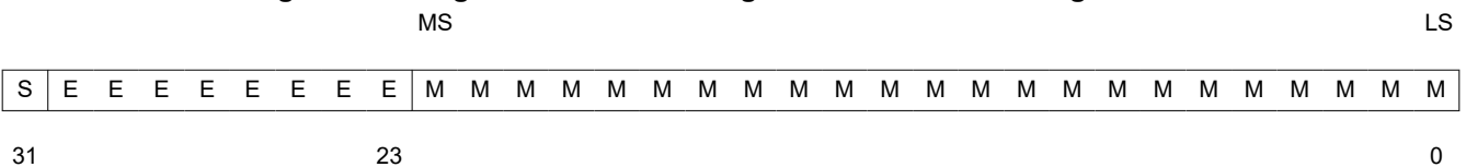
Figure 8-3. Single-Precision Floating-Point Char Data Storage Format
