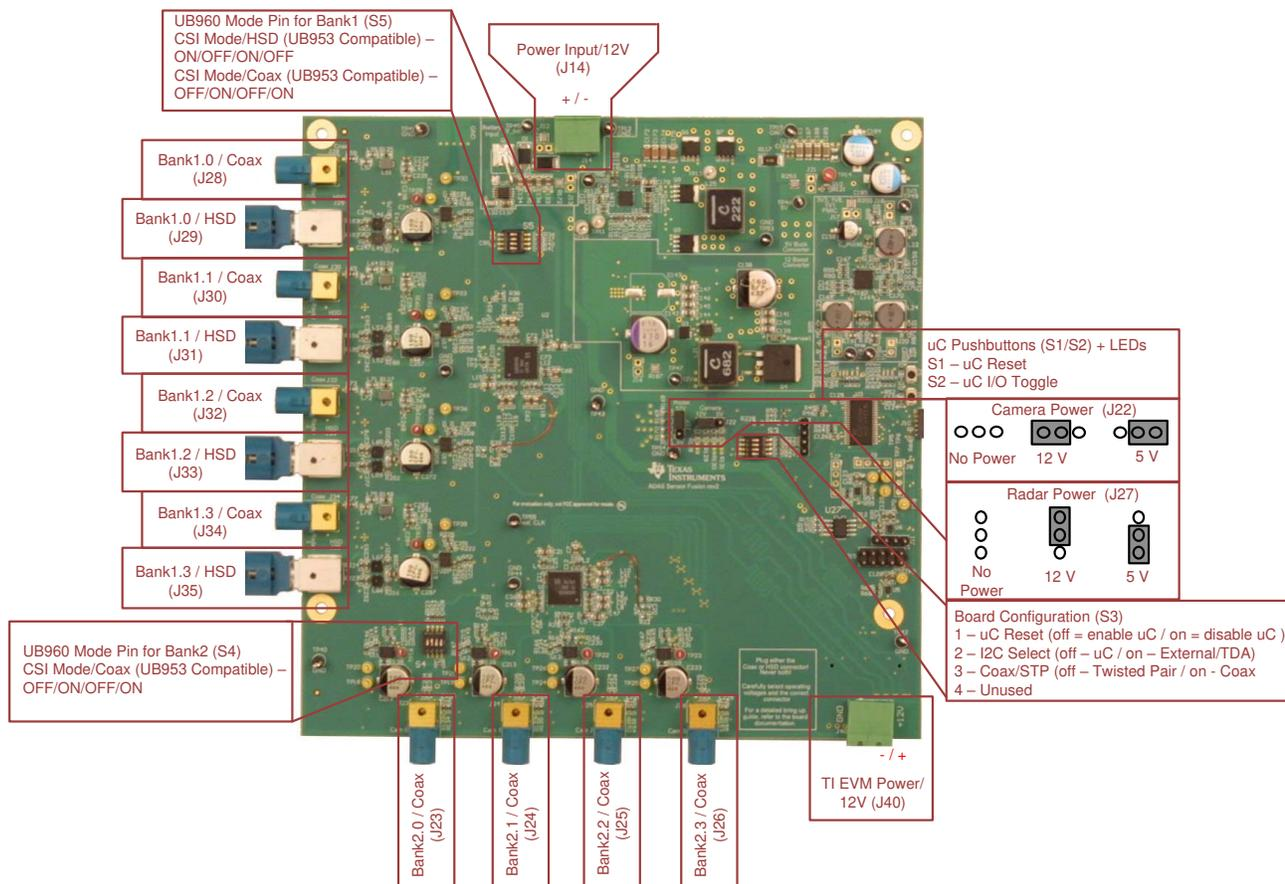
**Figure 3. Board With Components Identifications**
