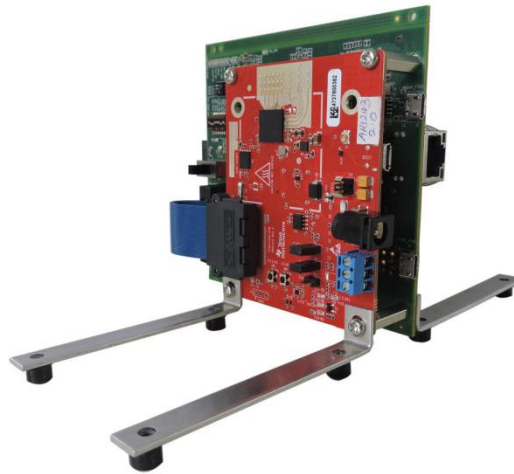
Figure 8. Connect Ribbon Cable (Side)
