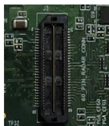
Figure 14. J3 High Density Interface Connector
