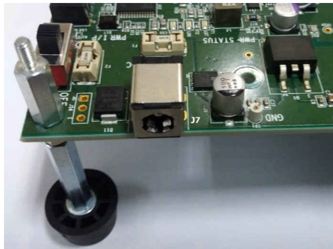
Figure 3-1. Connector Used for Power Input
