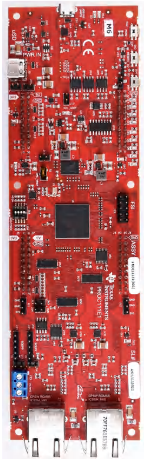
Figure 2-1. AM263x LaunchPad Board
