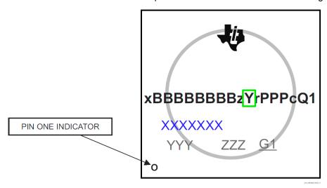
Figure 10-1. Printed Device Reference
