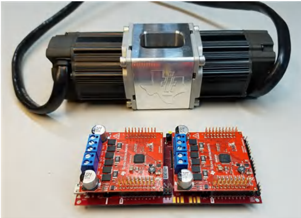
Figure 4. A Low-cost, Shunt-based Sensing Bundle for Motor-control Performance Testing
