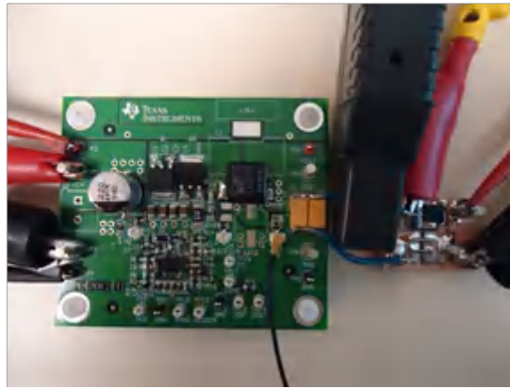
Figure 1-1. Typical Power-supply Test Setup for Fast Load Transient
