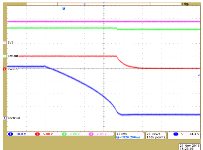
Figure 26. 30-V AC Shutdown
