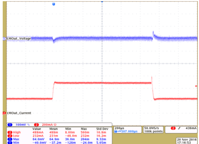
Figure 38. LM5166 Transient Response (200 to 480 mA)
