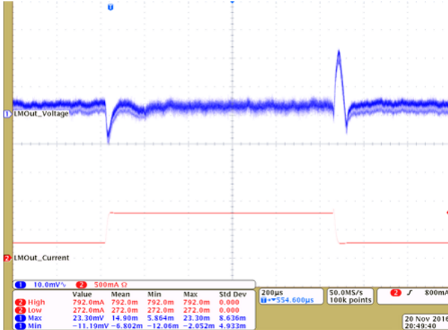
Figure 40. TLV61080 Transient Response (250 to 750 mA)
