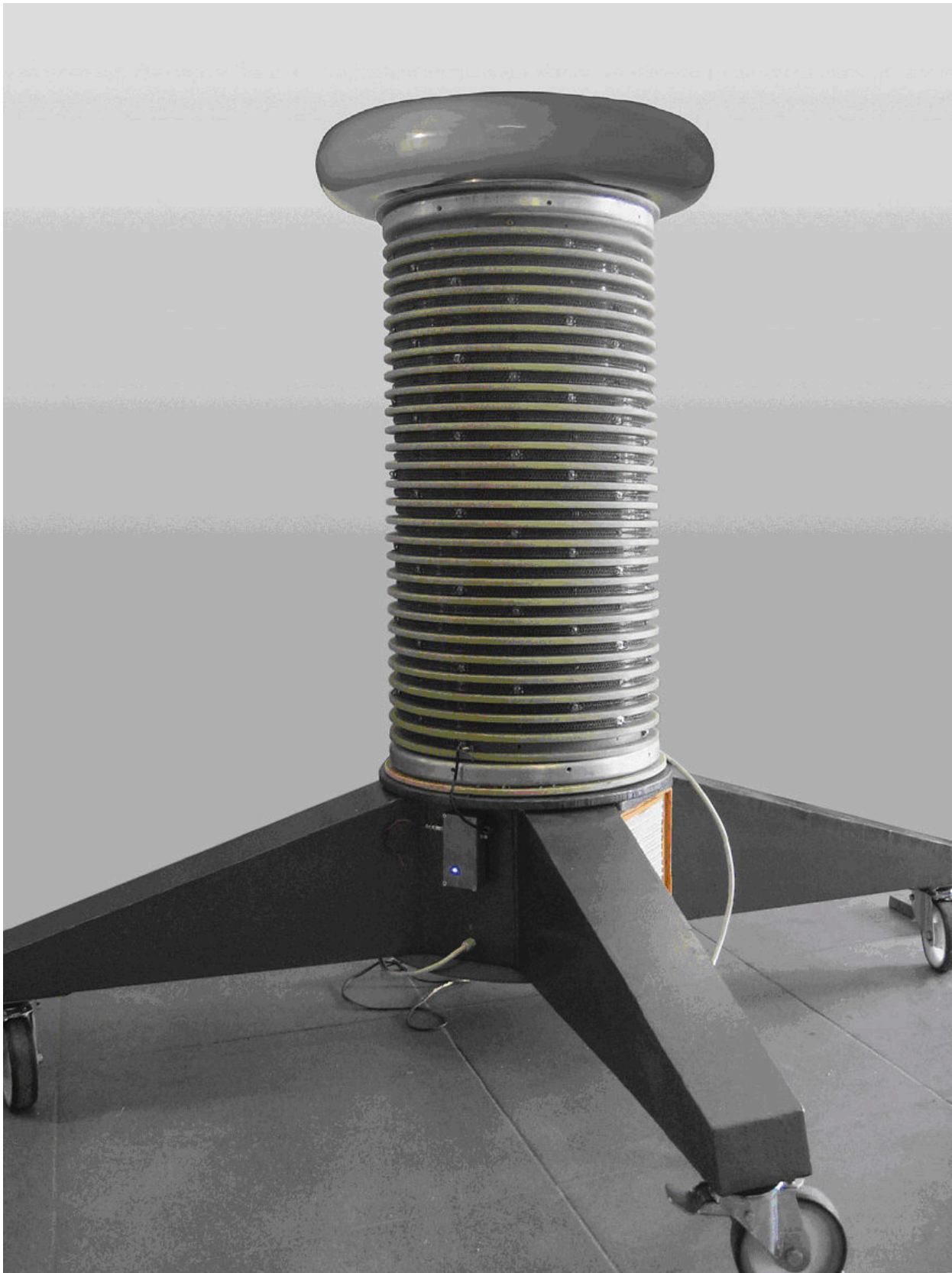
Figure 2-2. Common View of a 100-kV Reference Voltage Source
