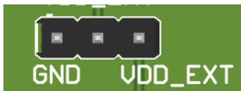
Figure 2-1. Header J2 : J2-1(GND), J2-2(Connection to device VDD), J2-3 (VDD_EXT)
