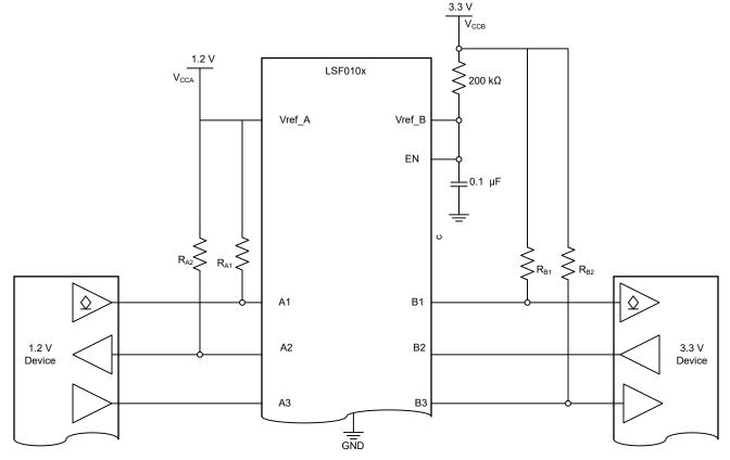
Figure 3-1. Example Schematic of LSF Used in Both Push-Pull and Open Drain Configurations
