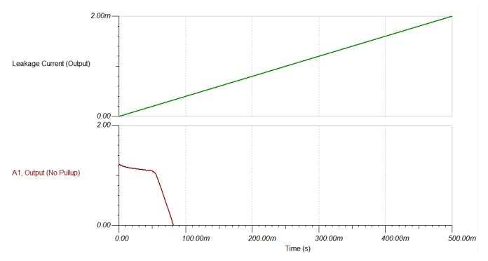
Figure 3-3. Simulation Result With Excessive Leakage on Receiver Side
