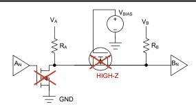
Figure 4-3. Leakage Current During an Input Logic High
