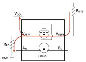
Figure 5-1. Using LDO Power Supply with LSF
