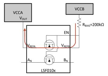
Figure 4-1. Leakage Current from Higher to Lower Power Supplies
