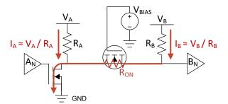
Figure 4-2. Leakage Current Into Driver Side During an Input Logic Low
