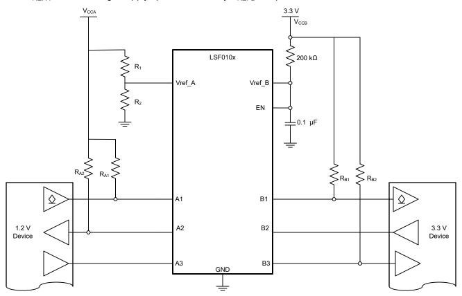
Figure 6-1. Voltage Divider Network on V<sub>REFA</sub>
