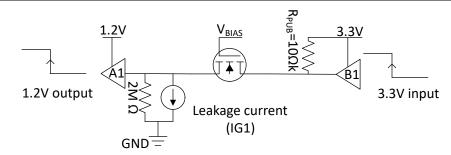
Figure 3-2. Simulation Setup With Excessive Leakage on Receiver Side
