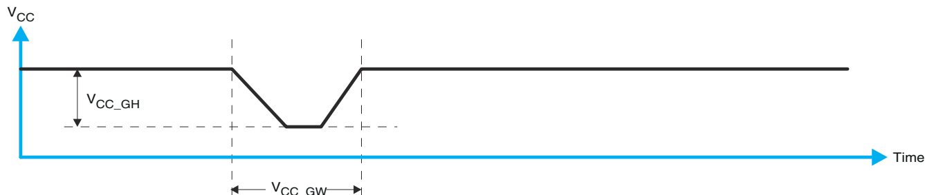
Figure 8-8. Glitch Width and Glitch Height
