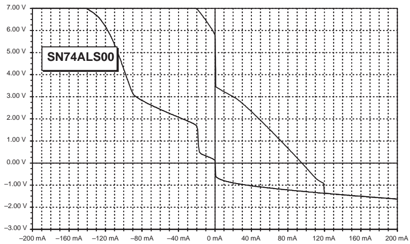
Figure 38. Output Characteristics of the SN74ALS00
