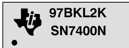
**Figure 2. Standard Marking**
