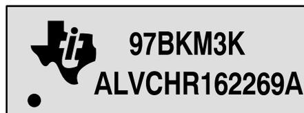
**Figure 3. Typical Abbreviated Device Marking**
