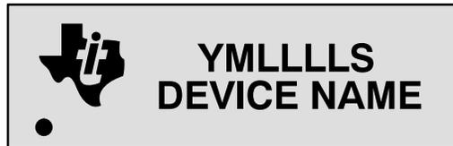
**Figure 5. Generic Marking Standard, Format 1**
