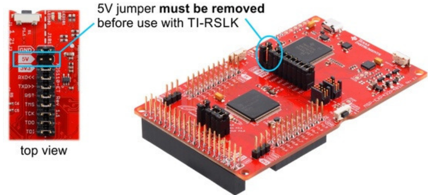
Figure 2b. TI MSP432 LaunchPad with headers pre-soldered and jumper removed.
