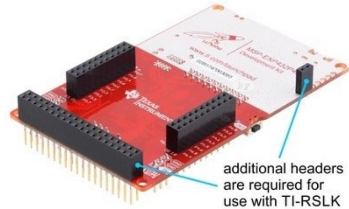
Figure 2a. TI MSP432 LaunchPad with headers pre-soldered .
