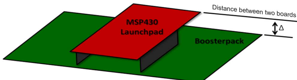
Figure 6. Connection of MSP430 LaunchPad and BoosterPack
