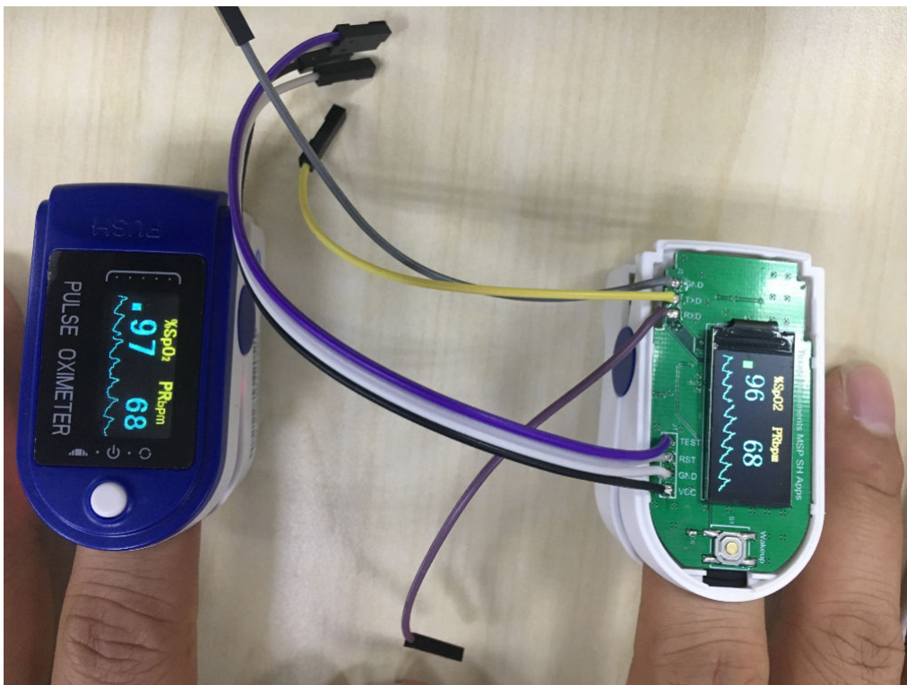
Figure 7-2. Comparison Test (Left: MP Pulse Oximeter, Right: Demo Base on FR2355)
