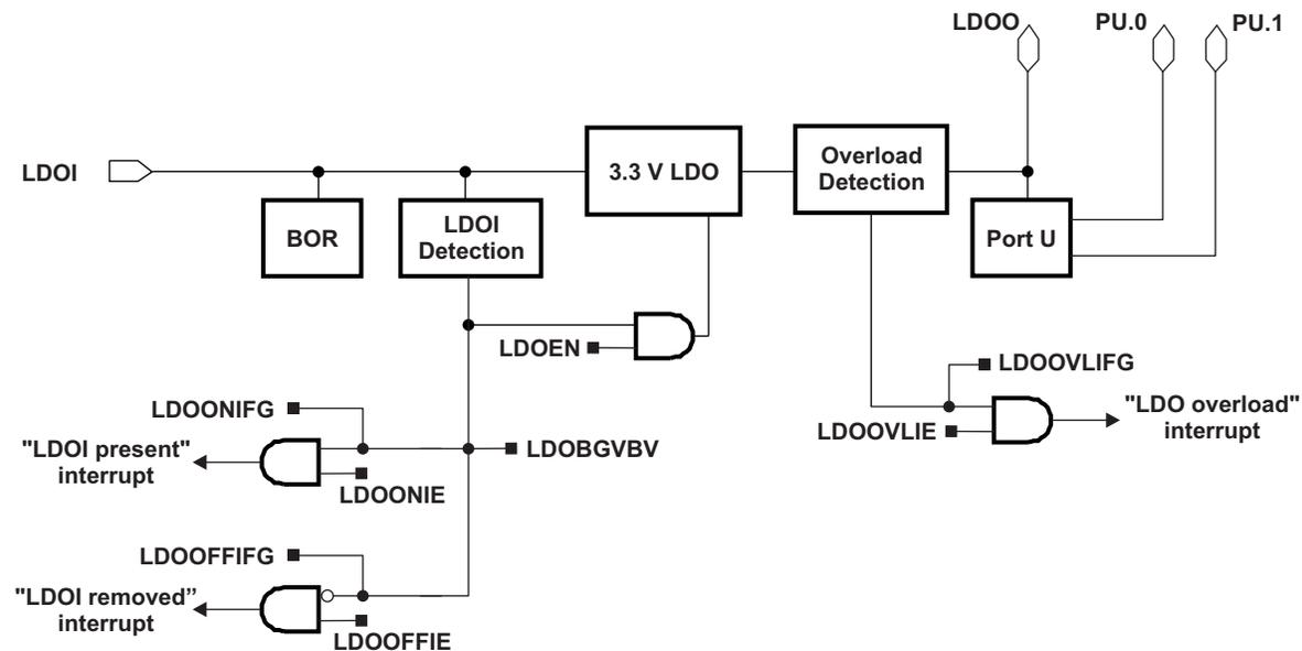
Figure 1-1. LDO Block Diagram
