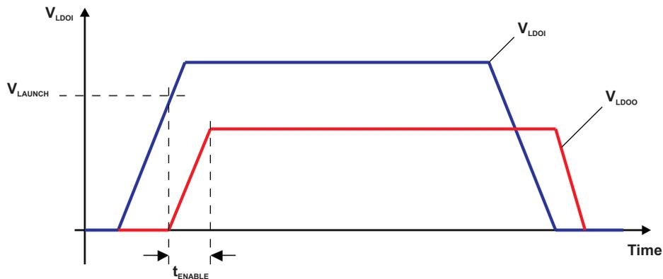
Figure 1-2. 3.3-V LDO Power Up/Down Profile
