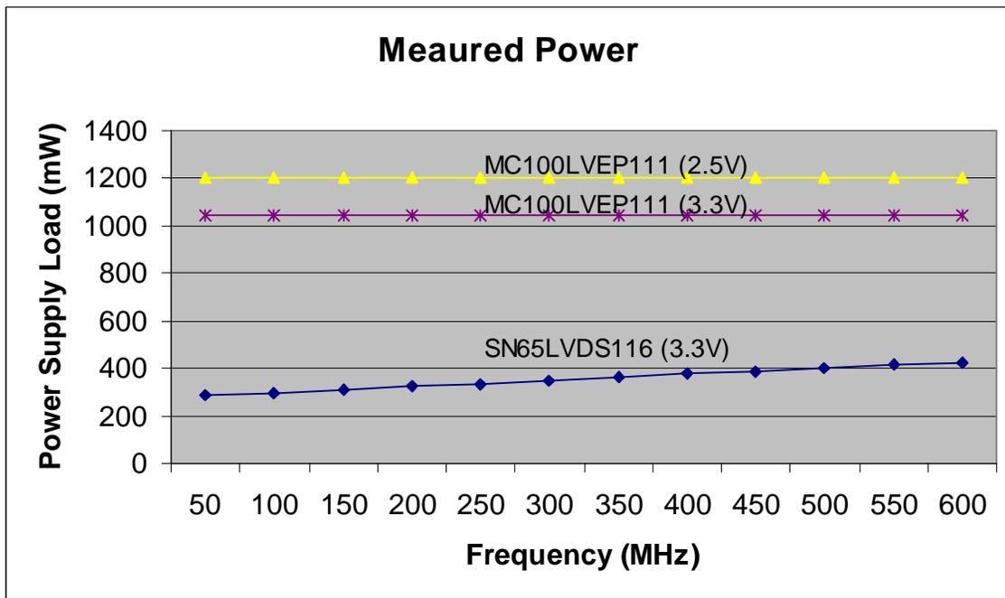
Figure 2. Measured Power
