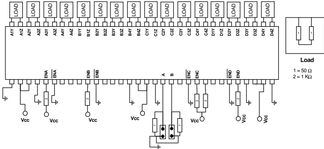
Figure 4. 1:16 LVDS Test Setup
