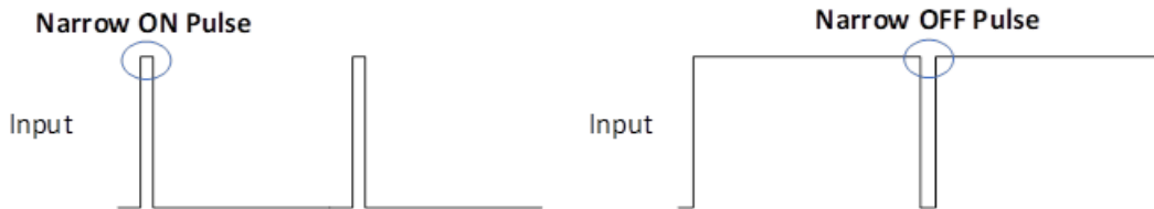
Figure 2-1. Narrow On Pulse and Narrow Off Pulse
