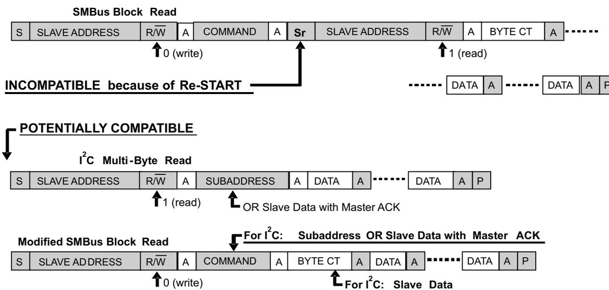
Figure 3. I<sup>2</sup>C Multi-Byte Read Compared to SMBus Block Read
