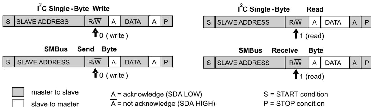
**Figure 1. I<sup>2</sup>C Single-Byte Write and Read Compared to SMBus Send and Receive Byte**
