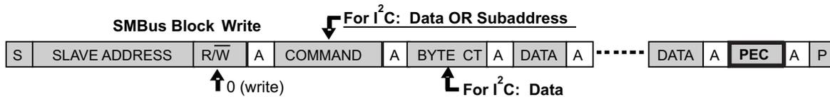
**Figure 4. SMBus Packet Error Checking (PEC)**
