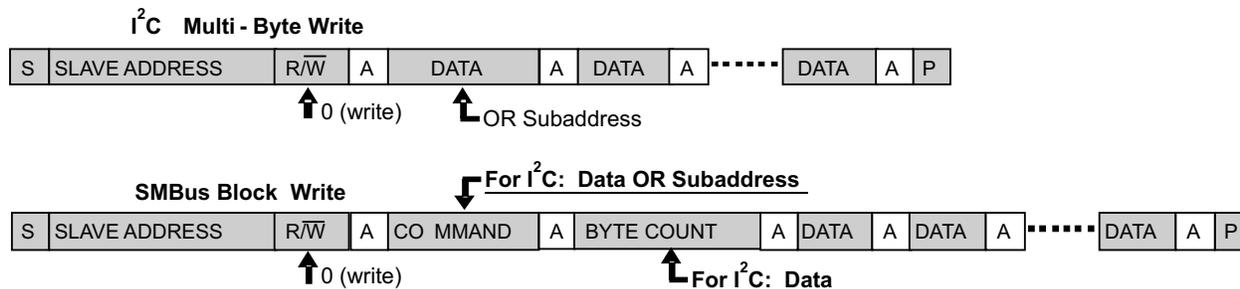
Figure 2. I<sup>2</sup>C Multi-Byte Write Compared to SMBus Block Write
