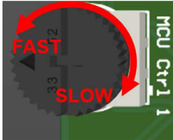
Figure 2-12. Speed Control Direction
