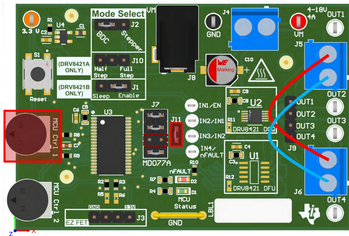
Figure 2-14. Parallel Mode Operation with DRV8421B
