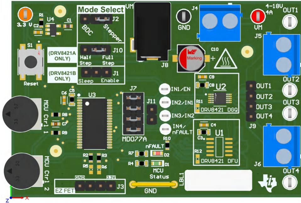
Figure 3-2. PCB (Top 3-D View)
