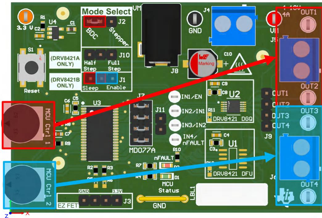
**Figure 2-11. EVM Controls for Brushed-DC Motor Operation with DRV8421B**
