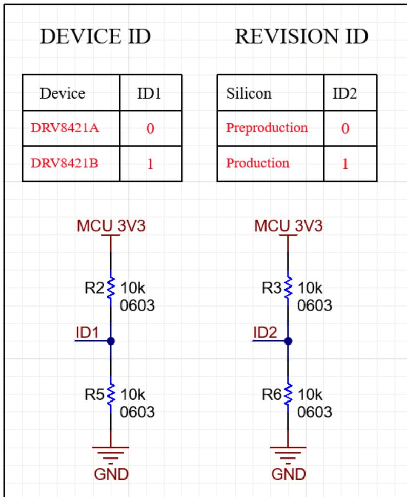
Figure 2-15. Device ID Resistors
