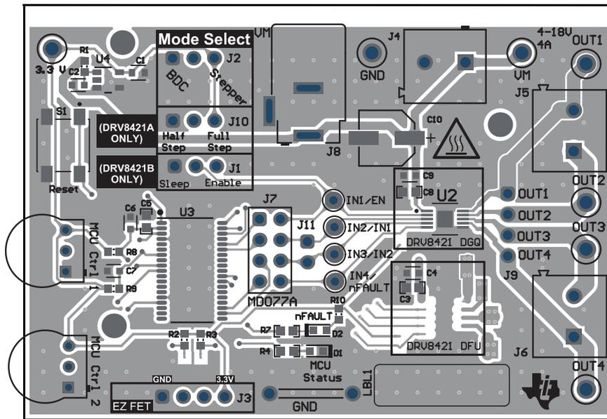
Figure 3-3. PCB (Top-Assembly View)
