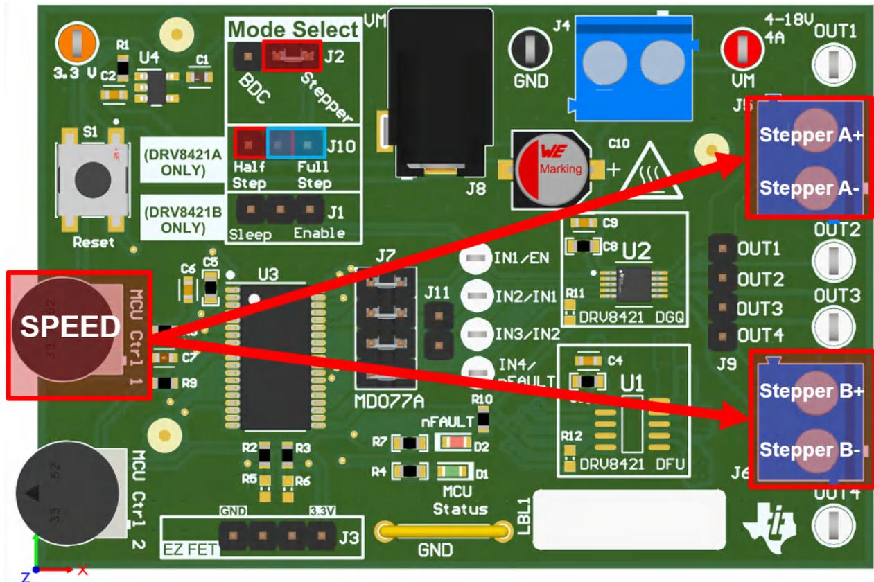
Figure 2-8. EVM Controls for Stepper Motor Operation with DRV8421A
