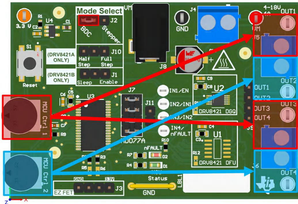
Figure 2-6. EVM Controls for Brushed-DC Motor Operation with DRV8421A
