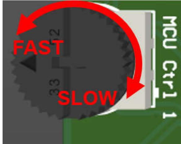
Figure 2-7. Speed Control Direction
