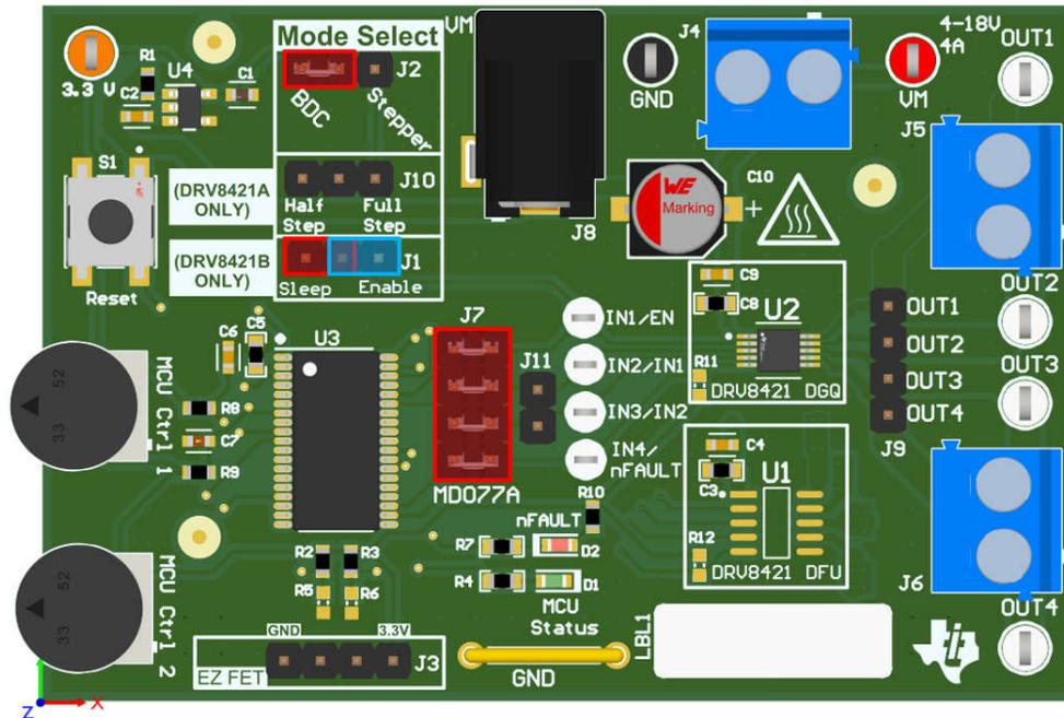
Figure 2-4. Jumper Configuration for Brushed-DC Motor Control with DRV8421B
