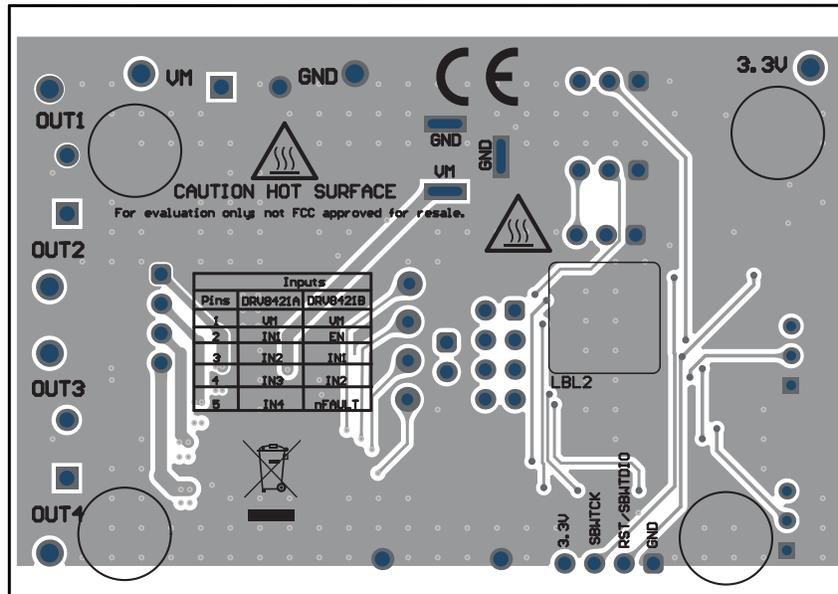
Figure 3-4. PCB (Bottom-Assembly View)
