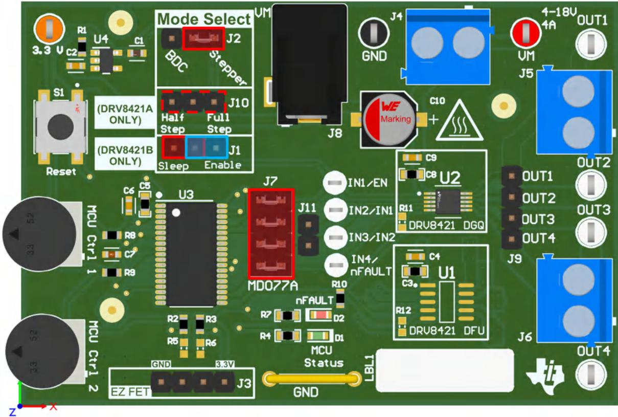
Figure 2-5. Jumper Configuration for Stepper Motor Control with DRV8421B
