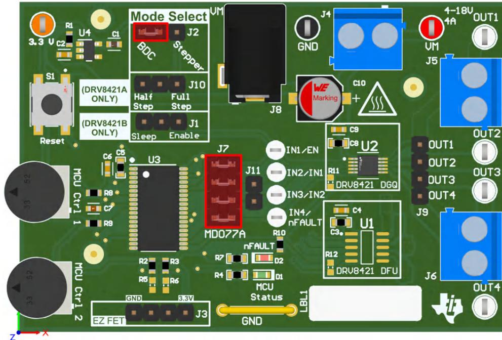
Figure 2-2. Jumper Configuration for Brushed-DC Control with DRV8421A
