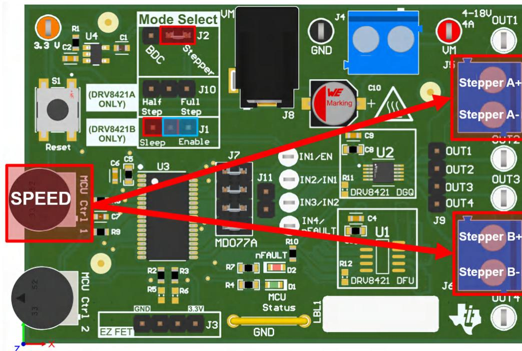
Figure 2-13. EVM Controls for Stepper Motor Operation with DRV8421B
