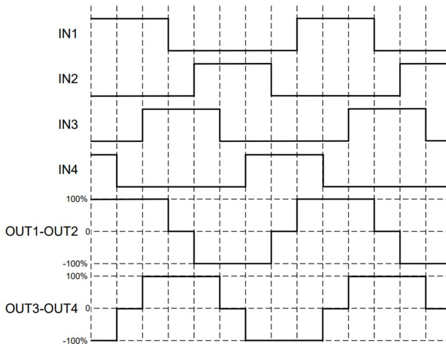
**Figure 2-10. Half-Step Sequence Waveforms**
