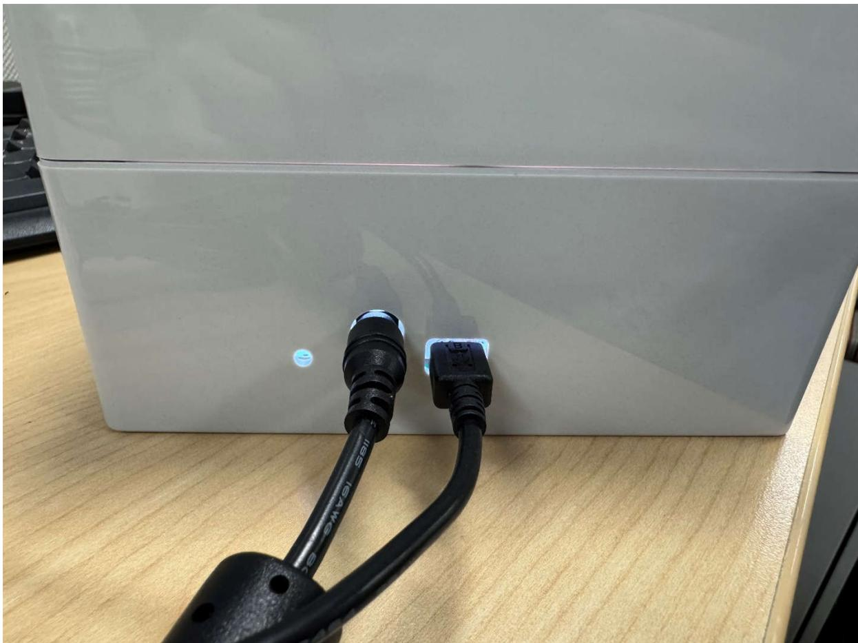
**Figure 2-1. USB and Power Connections**
