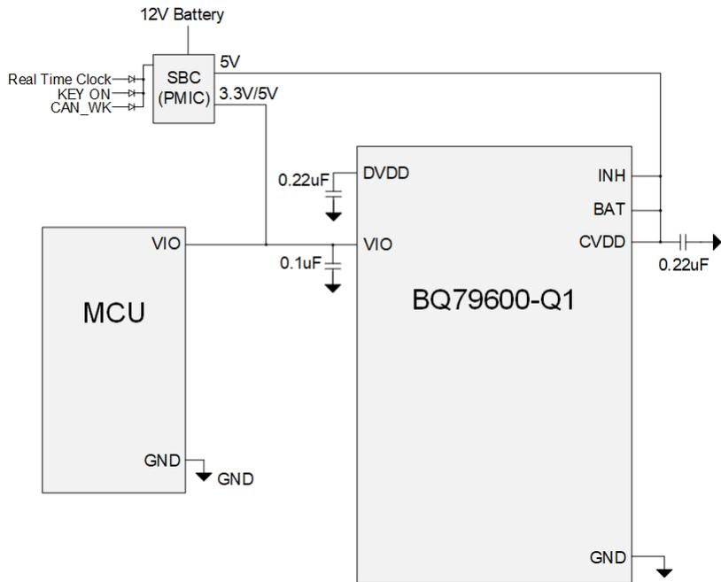
**Figure 1-2. 5 V Regulated Supply and No Automatic Host Wakeup**
