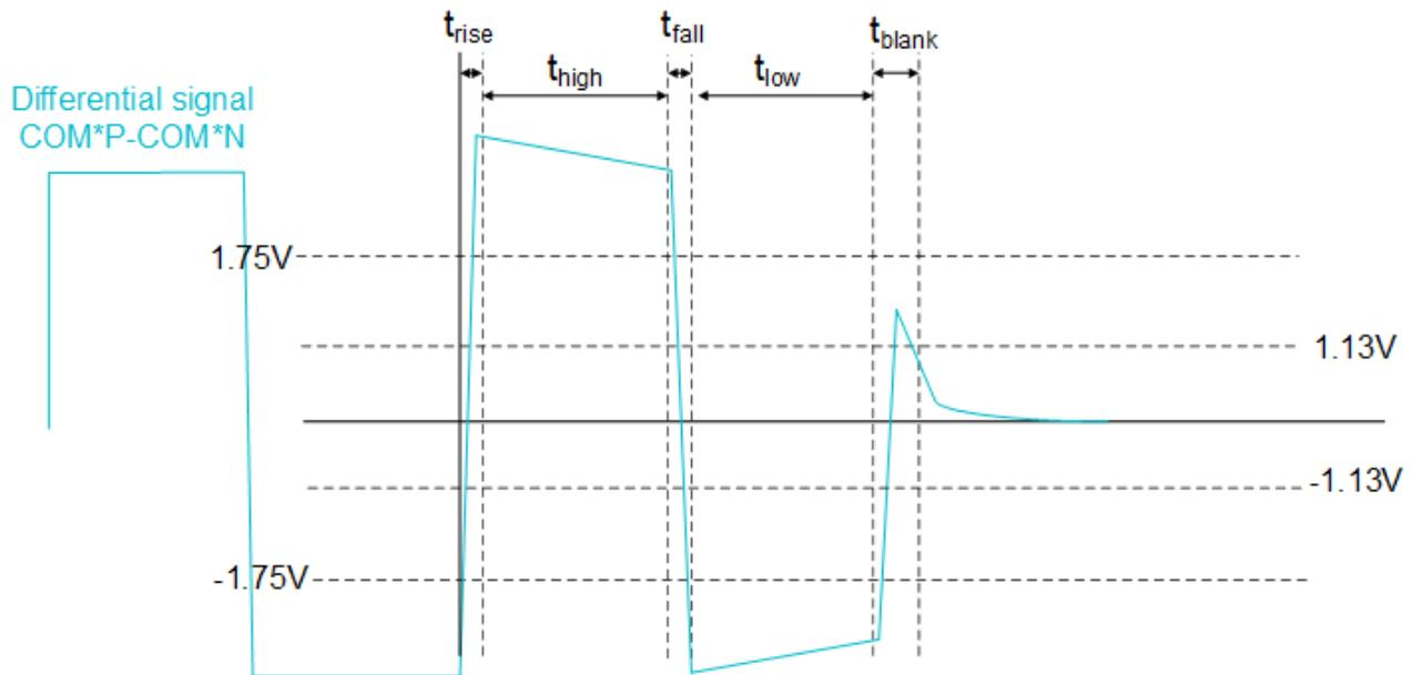
Figure 3-1. Daisy-chain Receiver Threshold
