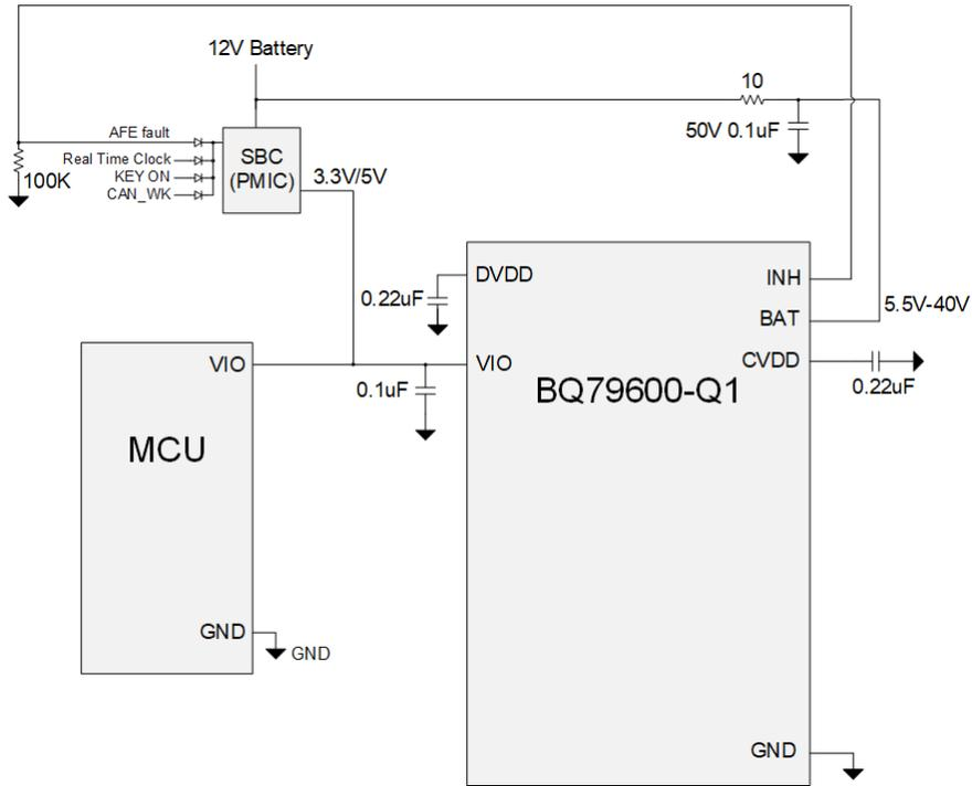
**Figure 1-1. 12 V Battery and Automatic Host Wakeup**
