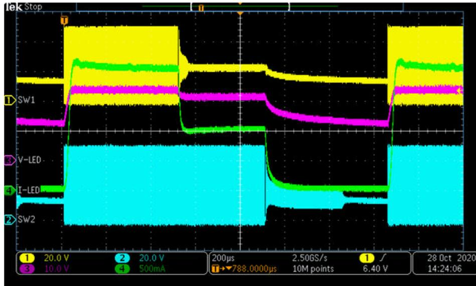
CH1-SW1 voltage, CH2=SW2 voltage, CH3-VLED voltage, and CH4 is ILED current.
