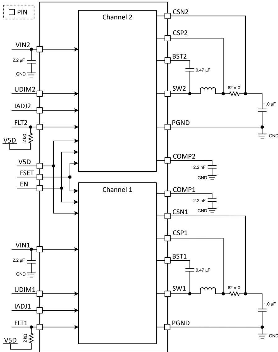
Figure 1-13. High Level Connections for TPS92519-Q1 Dual Synchronous Buck LED Driver
