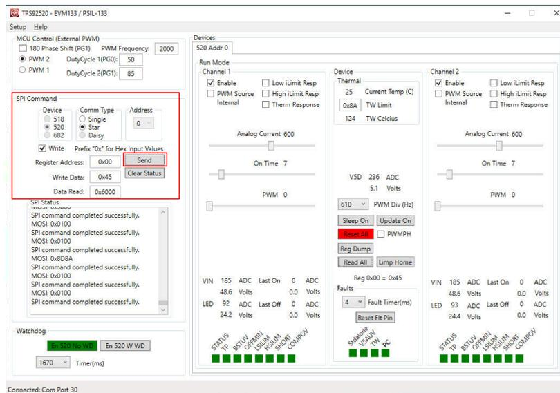
**Figure 1-9. Using GUI to Write 0x45h to SYSCFG1 Register at Address 0x00h**
