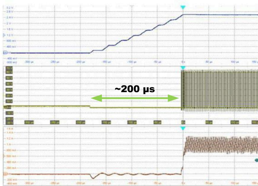
Figure 1-4. Start-up Waveform for a Single Channel
