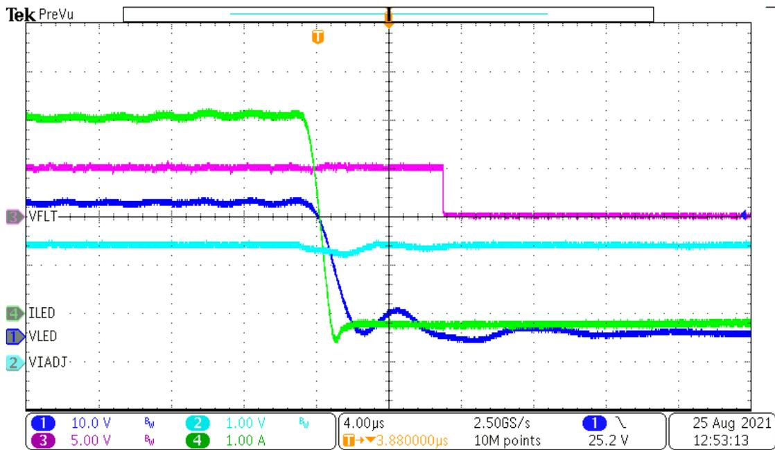
**Figure 1-18. Parallel Channels Exposed to Short Circuit Condition Using Modified TPS92519EVM-169**
