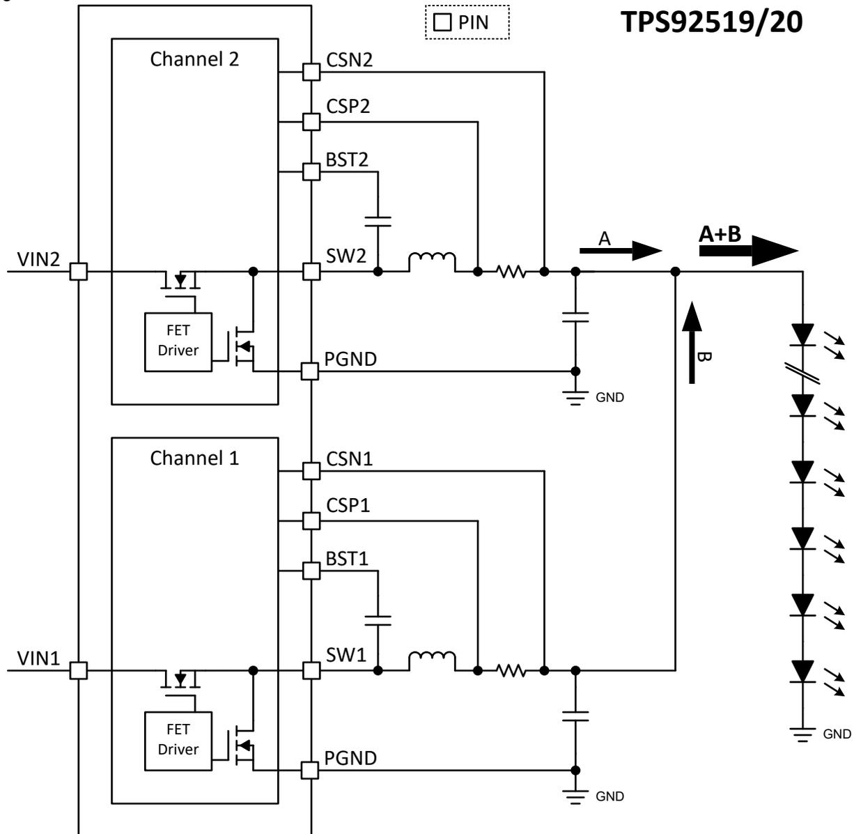
Figure 1-1. Dual Channel LED Driver Connected in Parallel - TPS92519-Q1 and TPS92520-Q1
