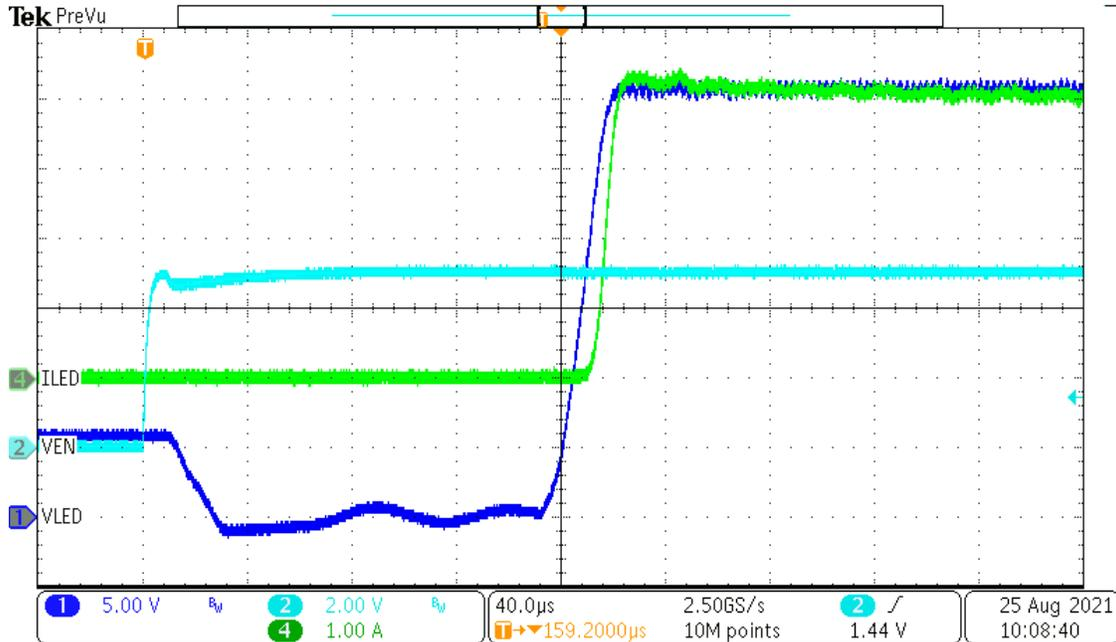
Figure 1-16. Parallel Channels Start-up Using Modified TPS92519EVM-1
