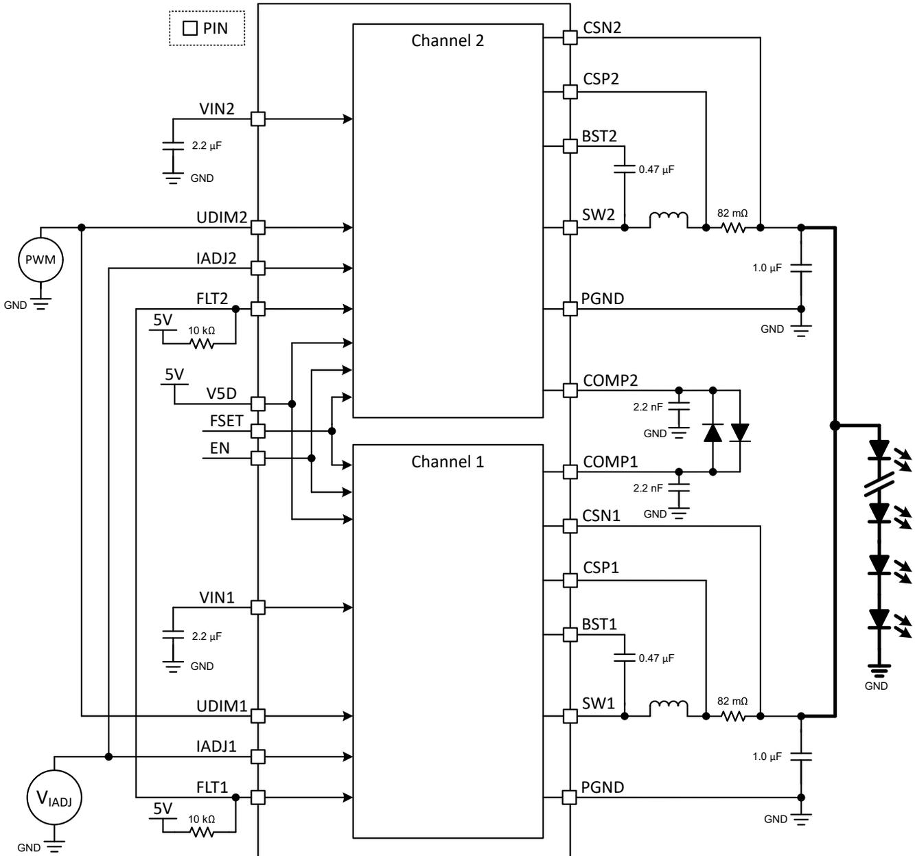
Figure 1-14. TPS92519-Q1 Connections Needed to Support Parallel Channel Operation
