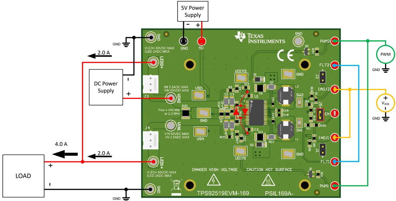
Figure 1-15. Connecting TPS92519EVM-169 for Parallel Operation
