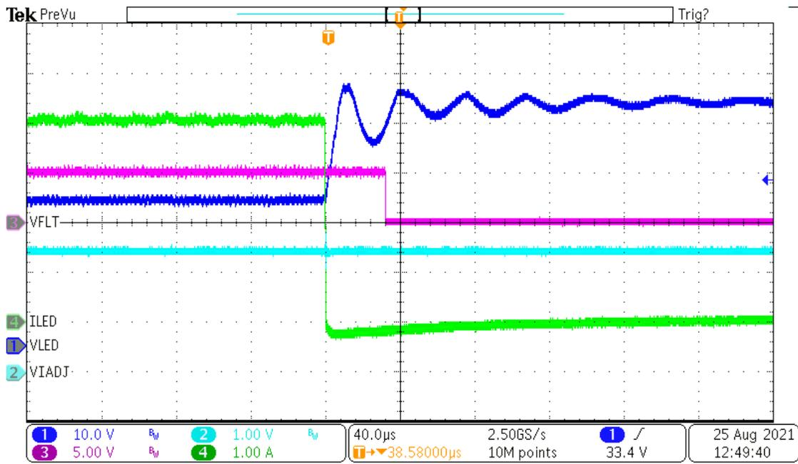
Figure 1-19. Parallel Channels Exposed to Open Circuit Condition Using Modified TPS92519EVM-169
