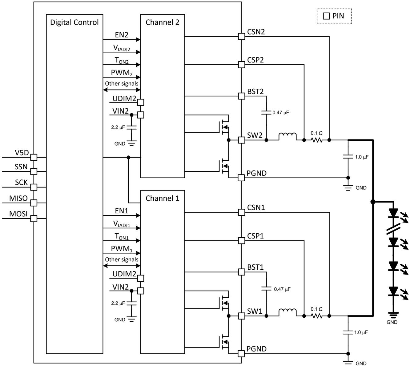
**Figure 1-2. High level Connections for TPS92520-Q1 Dual Synchronous Buck LED Driver**
