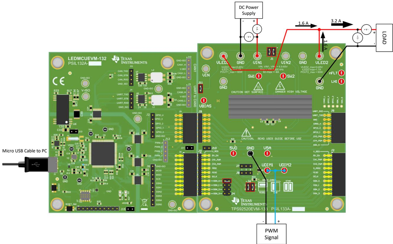
Figure 1-7. PWM Dimming Using External Signals to UDIM1 and UDIM2 Pins
