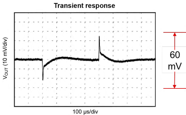
Figure 21. Feedthrough capacitor transient response.
