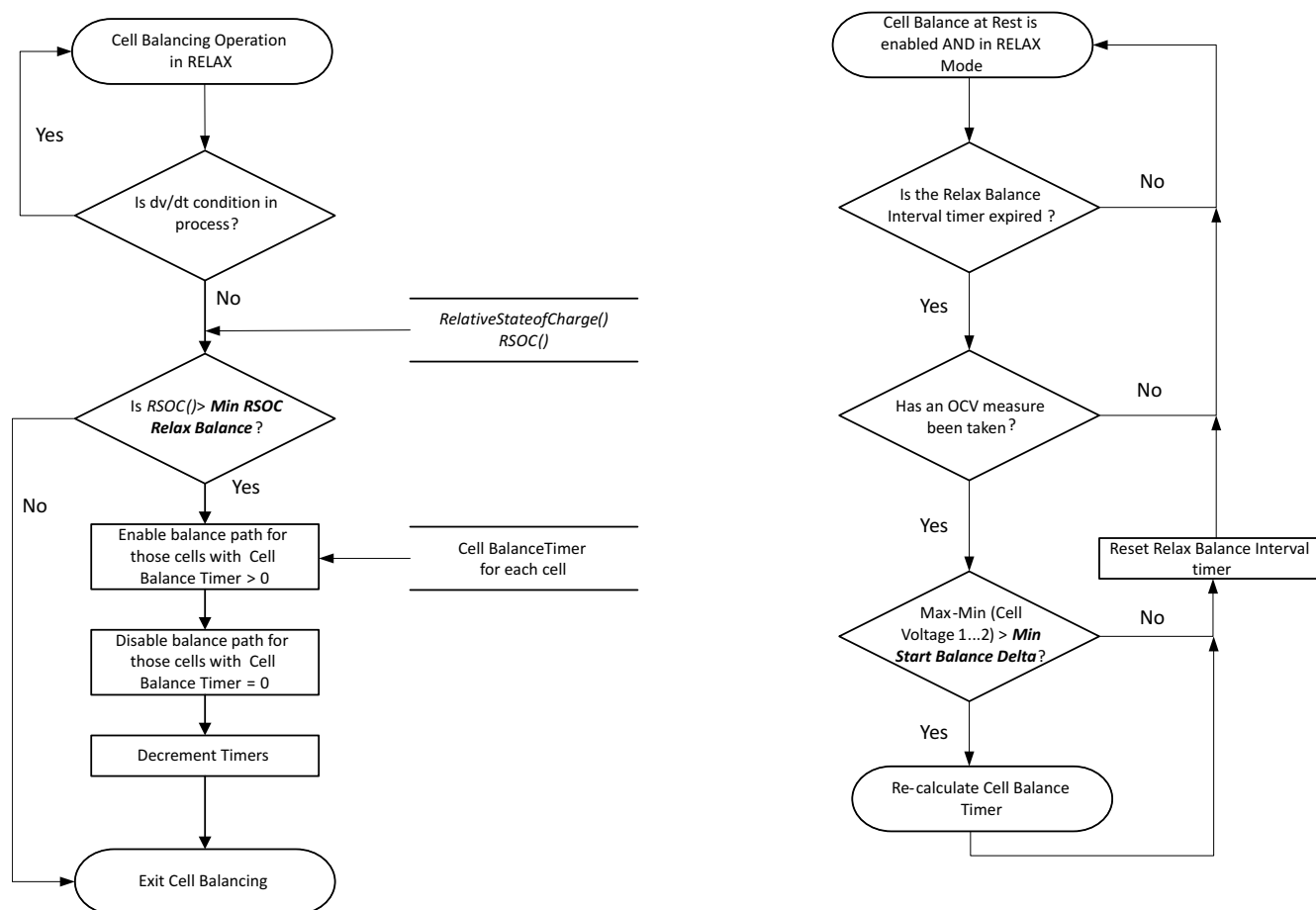
Figure 7-5. Cell Balance Operation in RELAX Mode
