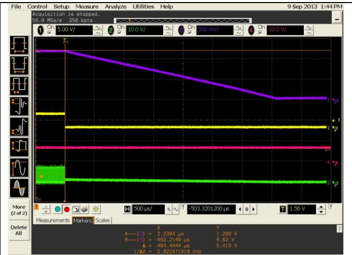
Figure 7 Turn-off, 7Vin, 1.2Vout, 10% of Rated Current
