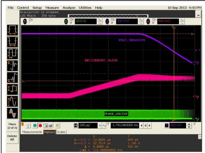
Figure 54 7Vin, 1.2Vout, Load regulation and over-current protection
