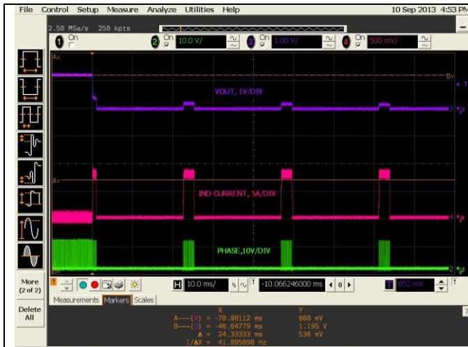
Figure 56 8Vin, 1.2Vout, Short circuit applied
