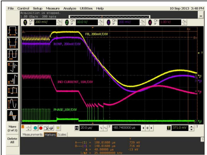
Figure 61 7Vin, 1.2Vout, Over-Voltage-Protection, Latch Off
