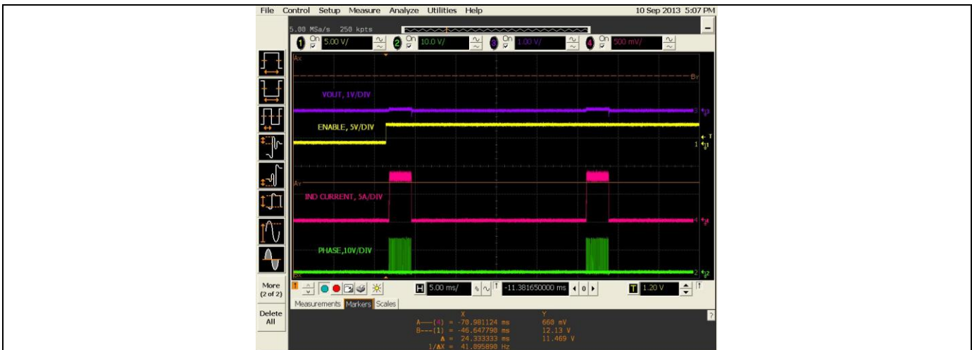
Figure 60 12Vin, 1.2Vout, Enable into short circuit
