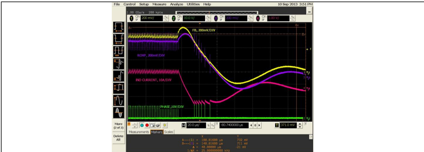
Figure 63 12Vin, 1.2Vout, Over-Voltage-Protection, Latch Off
