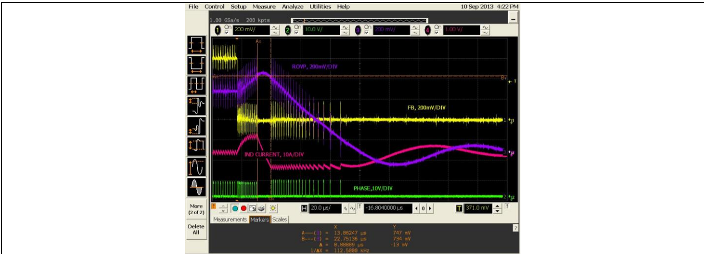
Figure 64 12Vin, 1.2Vout, FB shorted to GND
