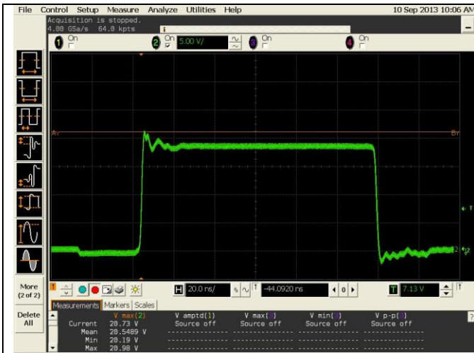
Figure 42 18Vin, 1.2Vout, 6A, Phase
