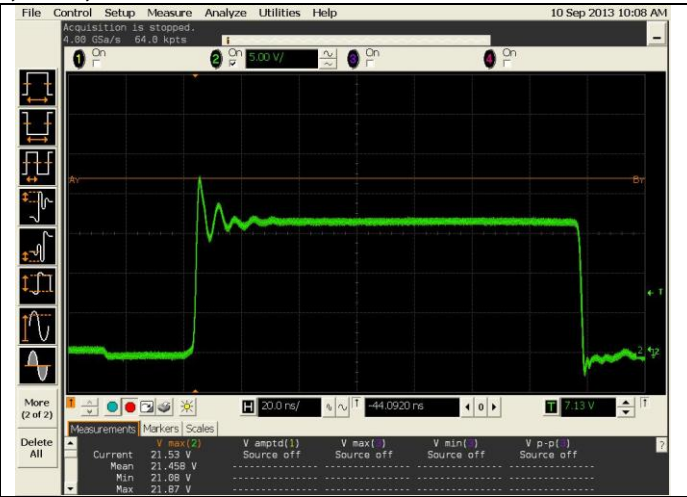
Figure 41 16Vin, 1.2Vout, 8A, Phase
