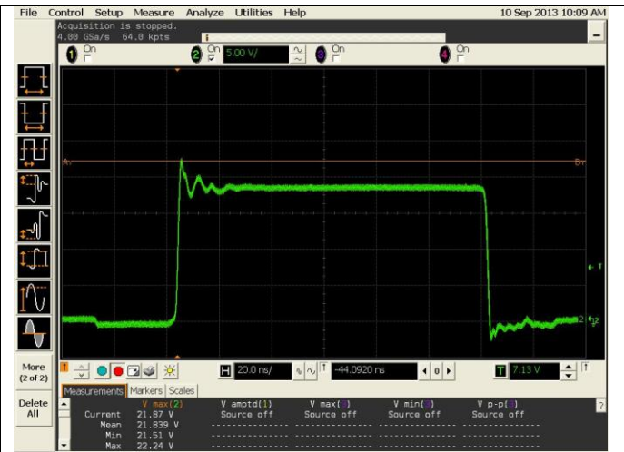
Figure 43 18Vin, 1.2Vout, 8A, Phase
