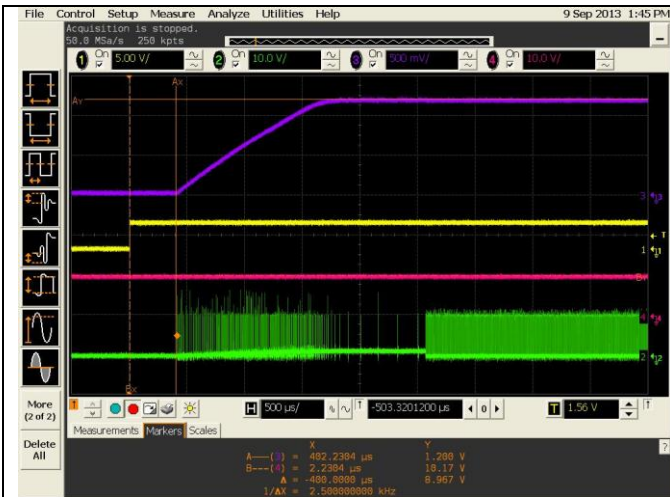
Figure 8 Turn-on, 10Vin, 1.2Vout, 10% of Rated Current
