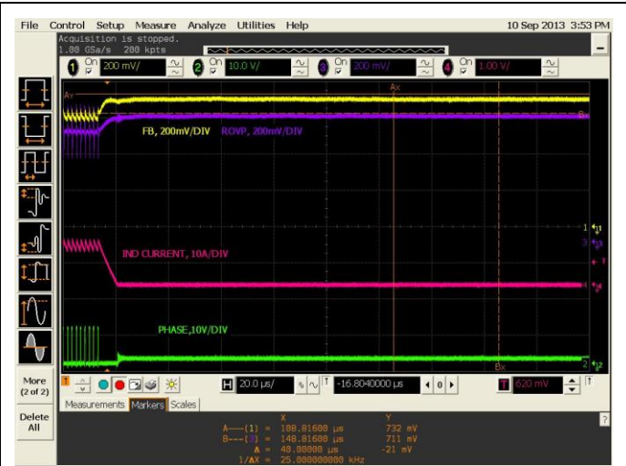
Figure 62 7Vin, 1.2Vout, Extreme transient response, No Latch
