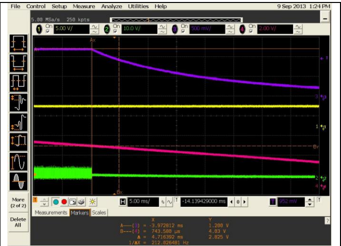
Figure 3 Turn-off, 10Vin, 1.2Vout, 10% of Rated Current
