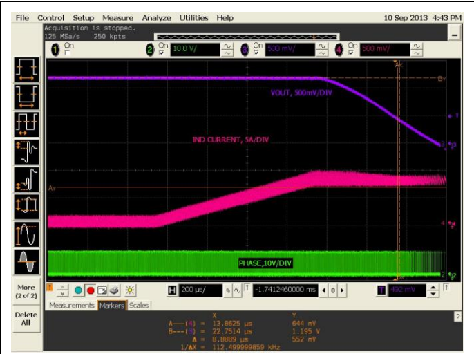
Figure 55 8Vin, 1.2Vout, Load regulation and over-current protection
