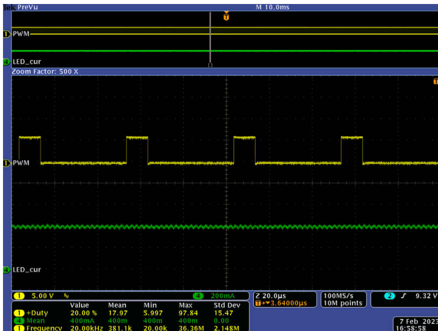
Figure 5-12. Waveforms at 20% Duty Cycle, 20 kHz Hybrid Dimming
