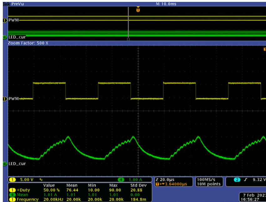
Figure 5-8. Waveforms at 50% Duty Cycle, 20 kHz PWM Dimming
