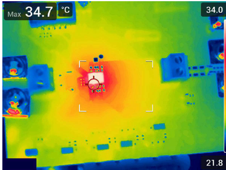
Figure 4-3. Thermal Performance (TPSM8287A10BAHEVM, V_{IN} = 5V , V_{OUT} = 0.9V , I_{OUT} = 10A )
