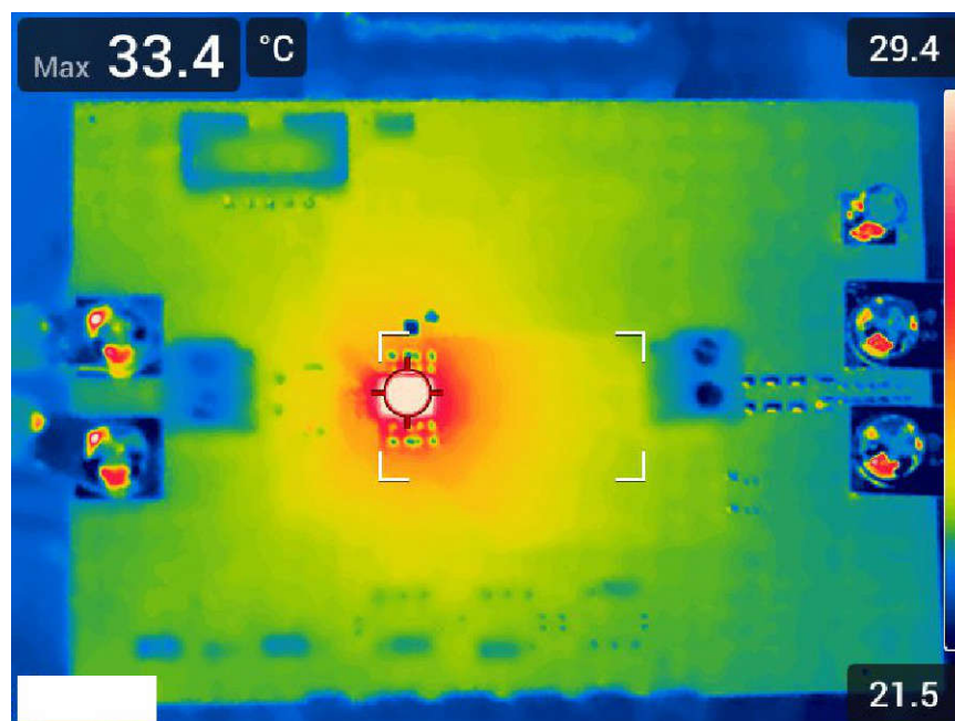
Figure 4-2. Thermal Performance (TPSM8287A06BASEVM, V_{IN} = 5V , V_{OUT} = 0.9V , I_{OUT} = 6A )
