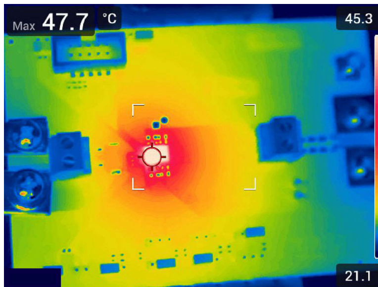
Figure 4-4. Thermal Performance (TPSM8287A15BBHEVM, V_{IN} = 5V , V_{OUT} = 0.9V , I_{OUT} = 15A )
