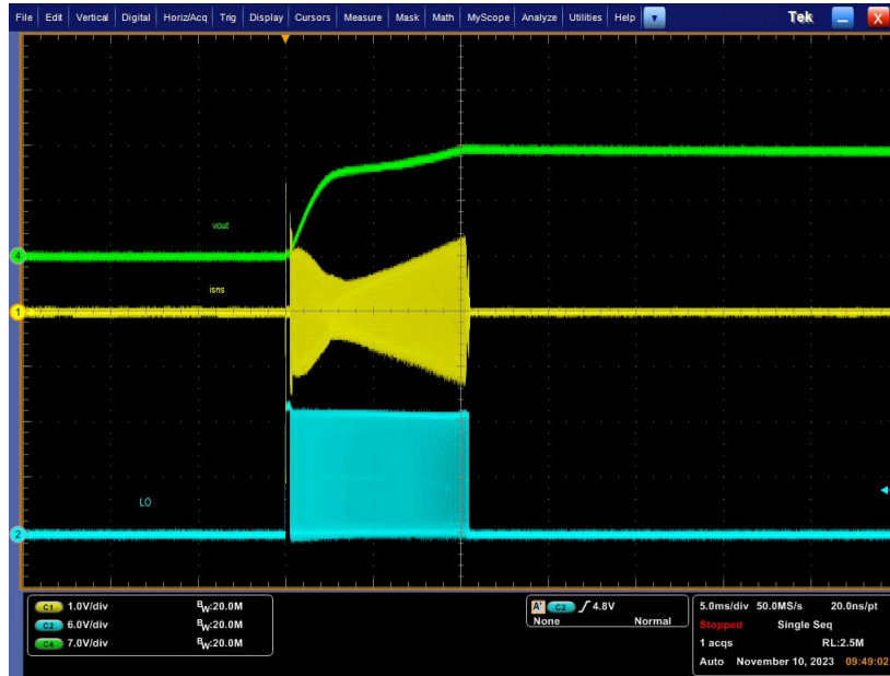
Figure 3-1. No Load (0 A) Startup (Ch1 = ISNS; Ch2 = LO; Ch4 = V OUT )
