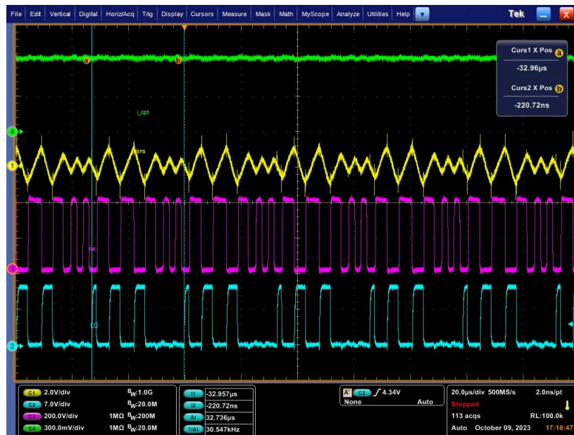
Figure 3-11. Steady State Waveforms at 1 A Load (Ch1= I SNS ; Ch2 = LO; Ch3 = SW; Ch4 = I OPT )
